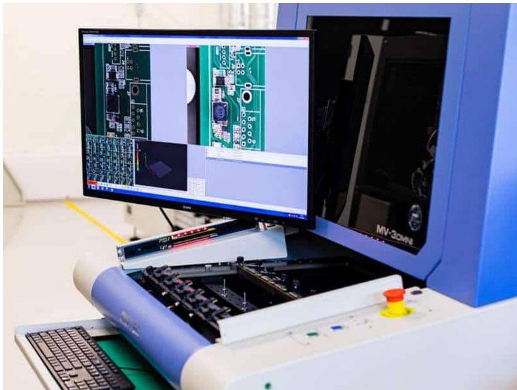
Figure 19 Automated Optical Inspection (AOI) [37]
