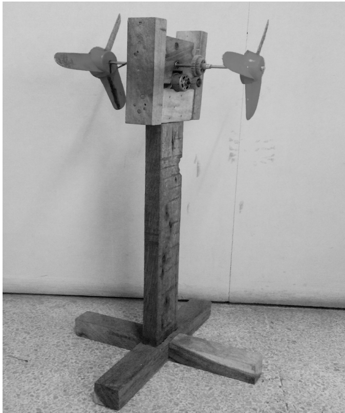
Fig. 3. Implemented multi-stage wind turbine.
