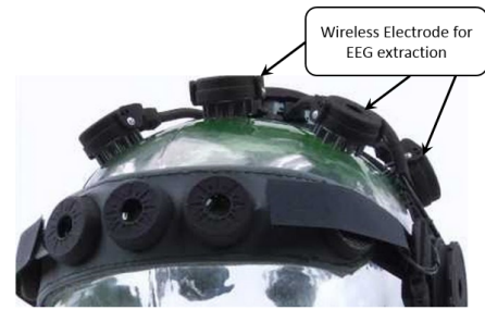
Fig. 4. A typical placement of dry electrode along scalp.
