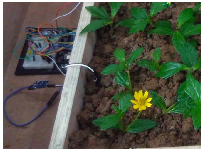
Fig 3: Setup of the Soil moisture Sensor
