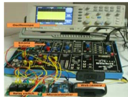
Fig 6. Experimental setup for Telecom Lab
