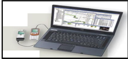
Fig. 4. Equipment setup during drive test
