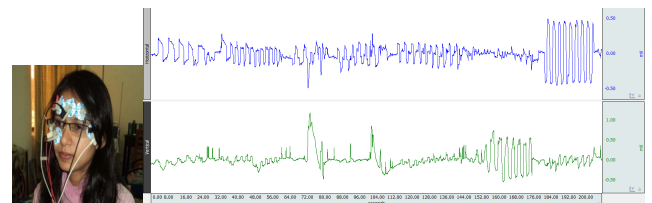
Fig. 8. EOG signal extraction and extracted raw EOG signal.
