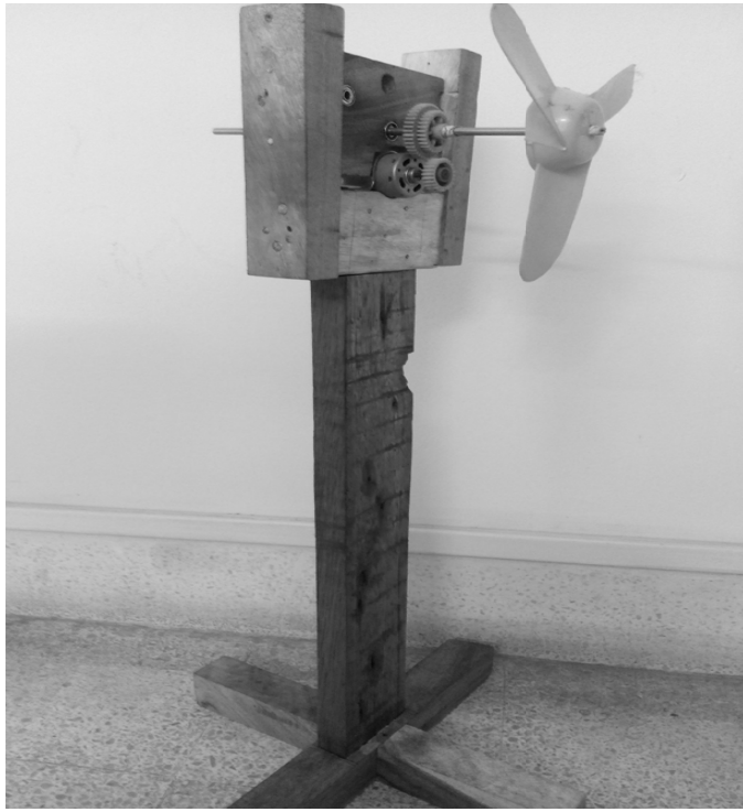
Fig. 2. Implemented single stage wind turbine.
