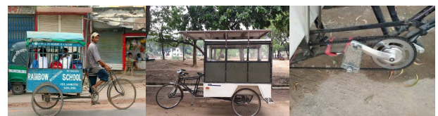
Fig. 1. Traditional rickshaw-van and rickshaw-van with PV array and torque sensor pedal installed
