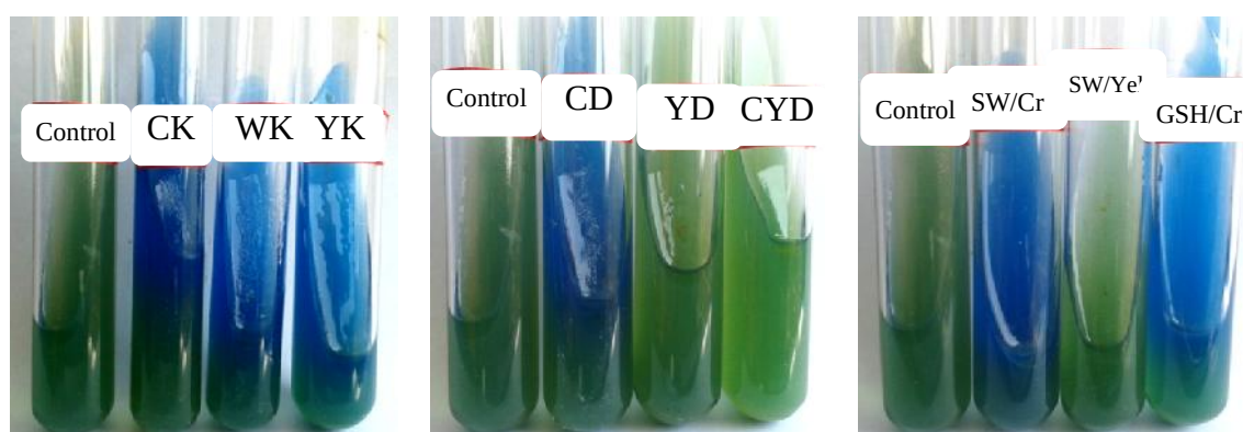
Plate 3.6 Bacterial isolates (N=9) along with control tube showing growth results in Simmons Citrate (SC) agar media.
