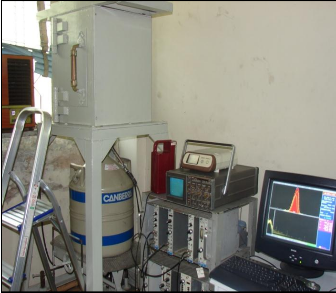
Figure-2.8: Canberra HPGe detector with digital \gamma -spectrometry system
