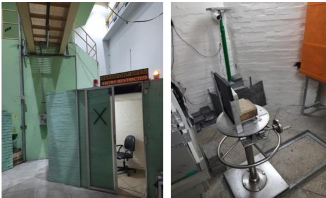
Figure-2.10: The Tangential beam port of TNRF at TRIGA Mark-II Research Reactor
