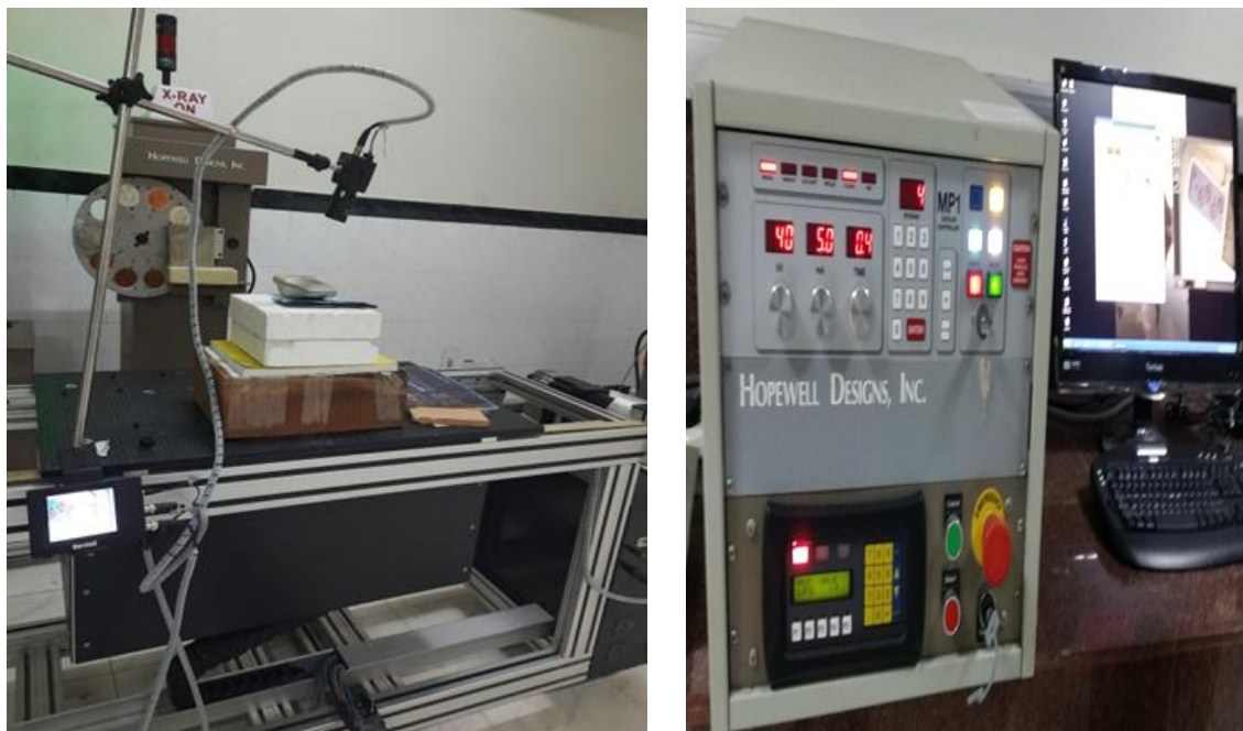
Figure-2.4: Experimental set-up and Control Panel of X-ray attenuation analysis
