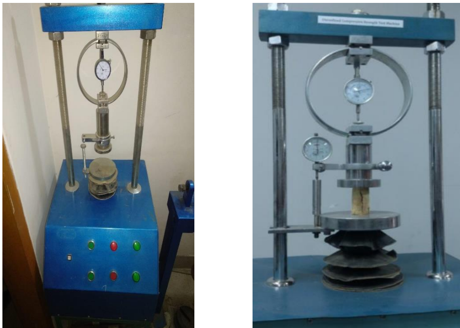
Figure 3-7: Unconfined Compression Test Machine.
