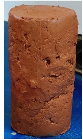
(a) (b) Figure 3-18: (a) Axial stress vs axial strain (b) failure mode of clay-2 at water content 35%.
