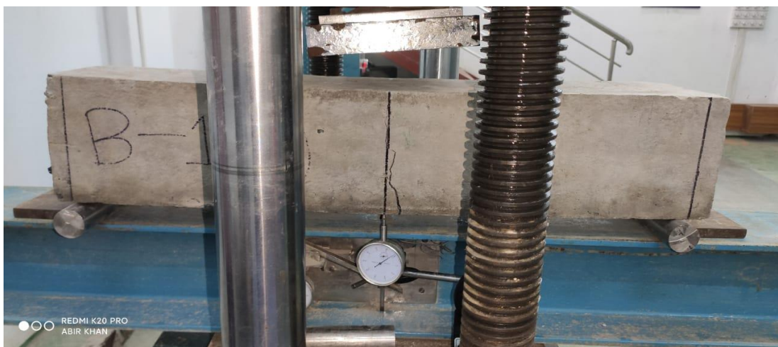
Figure 42: Failure pattern (for type 3 beam)
