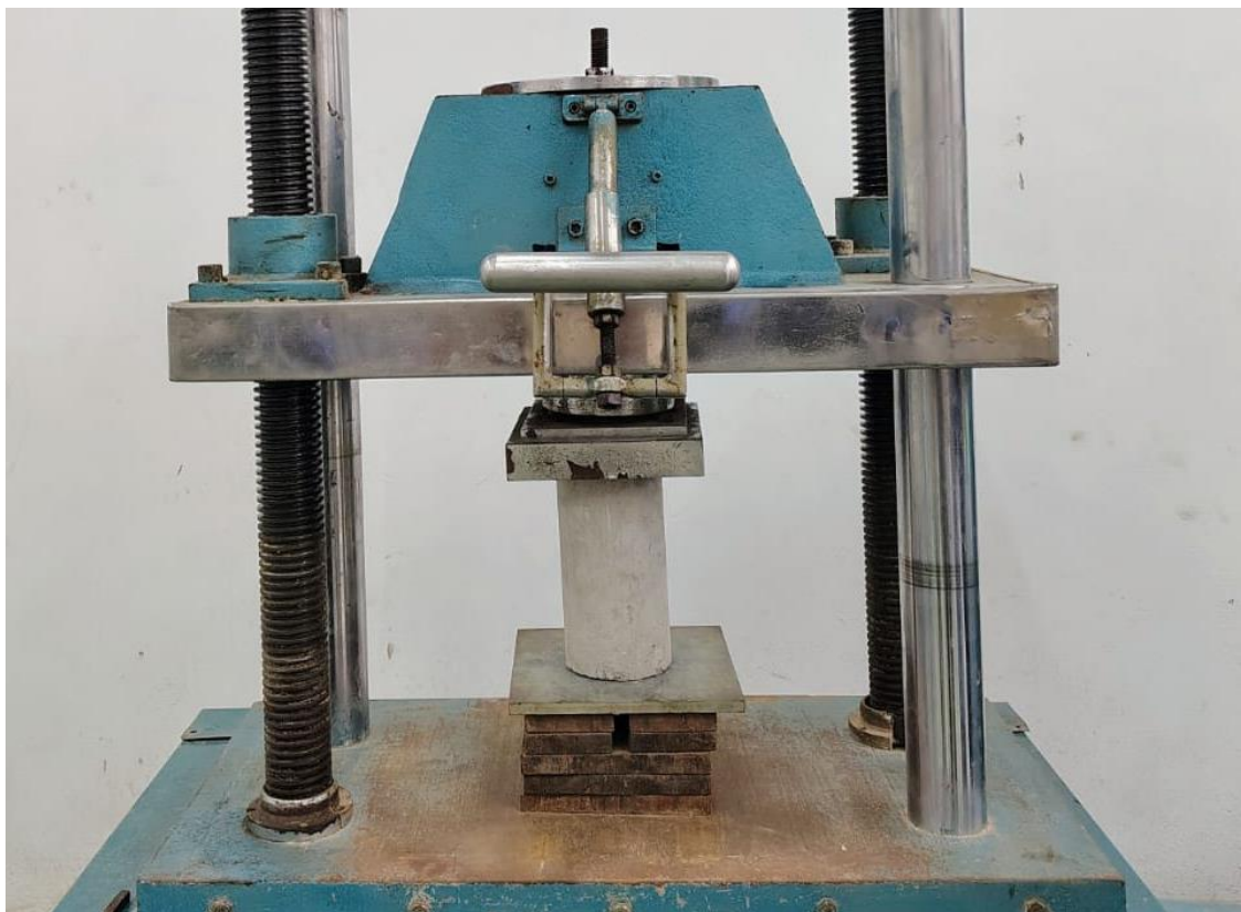
Figure 10: Setup of compressive strength test for slender
