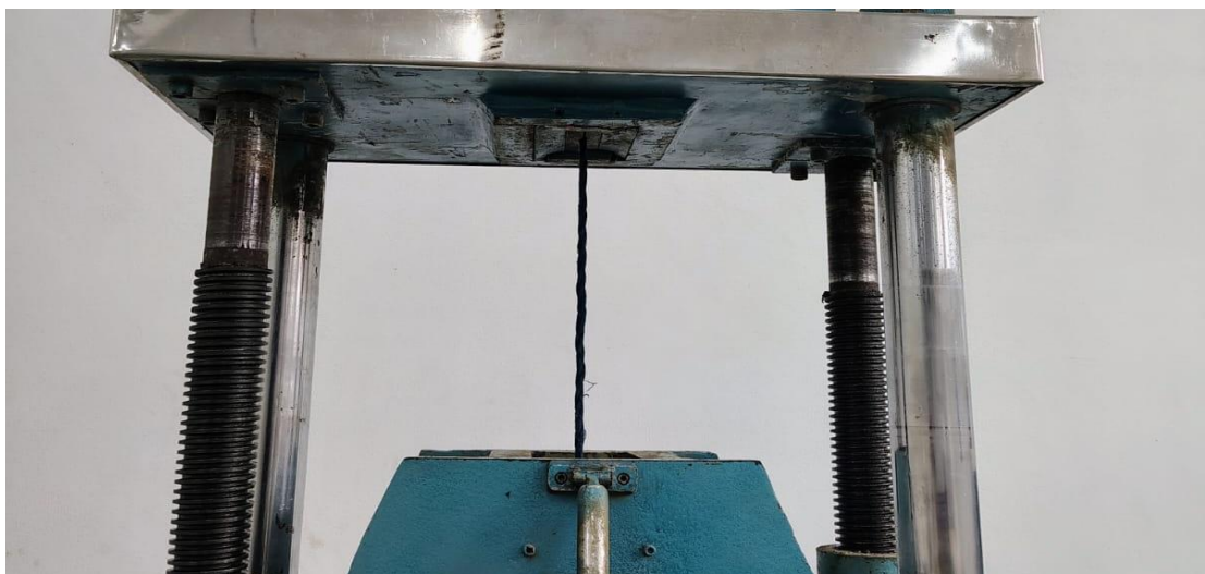
Figure 12: Setup for tensile test of textile reinforcement
