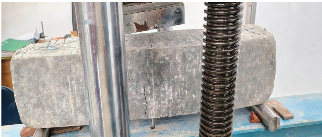
Figure 39: Failure pattern (for type 1 beam)
