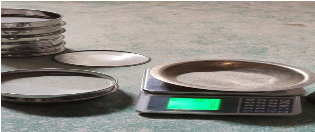
Figure 2: Fiennes modulus for fine aggregate
