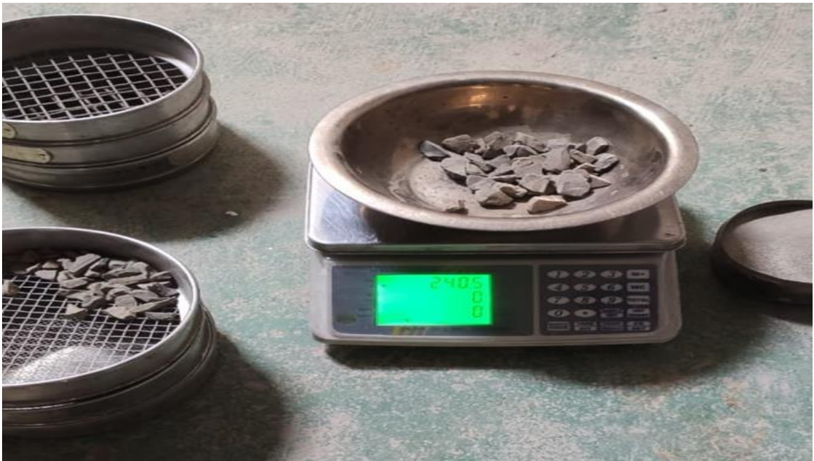
Figure 5: Fiennes modulus for coarse aggregate
