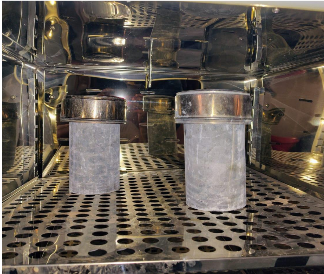
Figure 17: Oven-dry of specimen at 200°C for 1 hour
