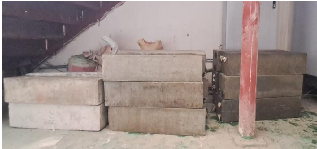
Figure 23: Beams after 28 days of curing
