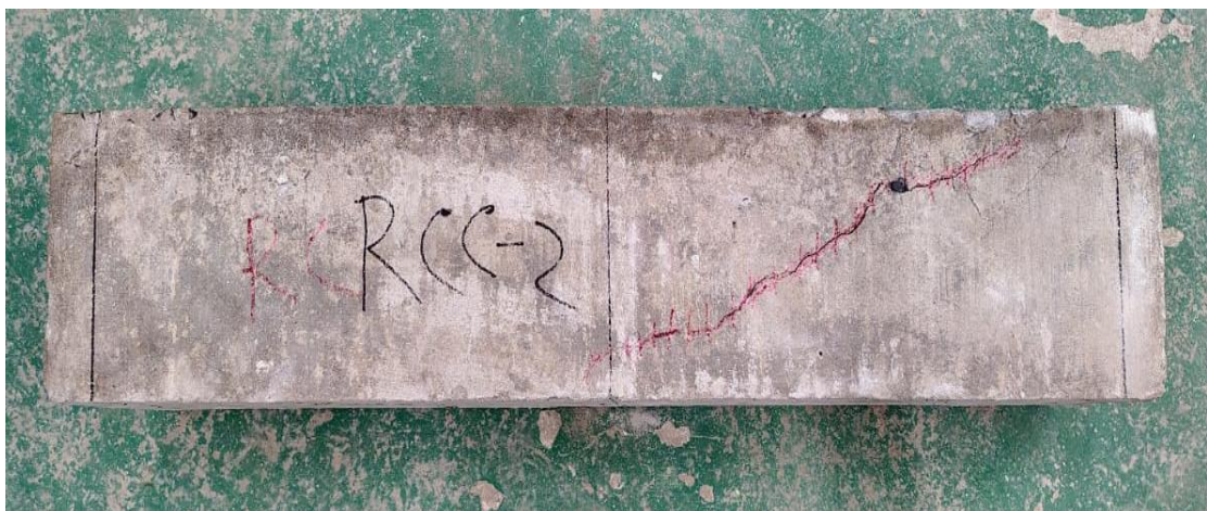
Figure 41: Failure pattern (for type 2 beam)
