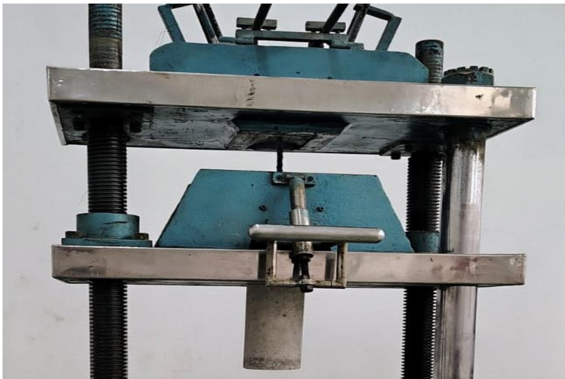
Figure 16: Setup of pull-out test for specimen
