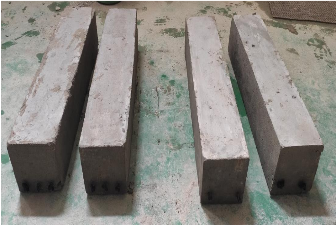
Figure 21: Beam two day after casting
