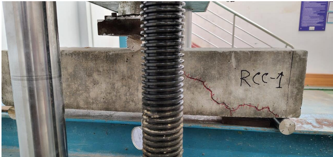
Figure 40: Failure pattern (for type 2 beam)
