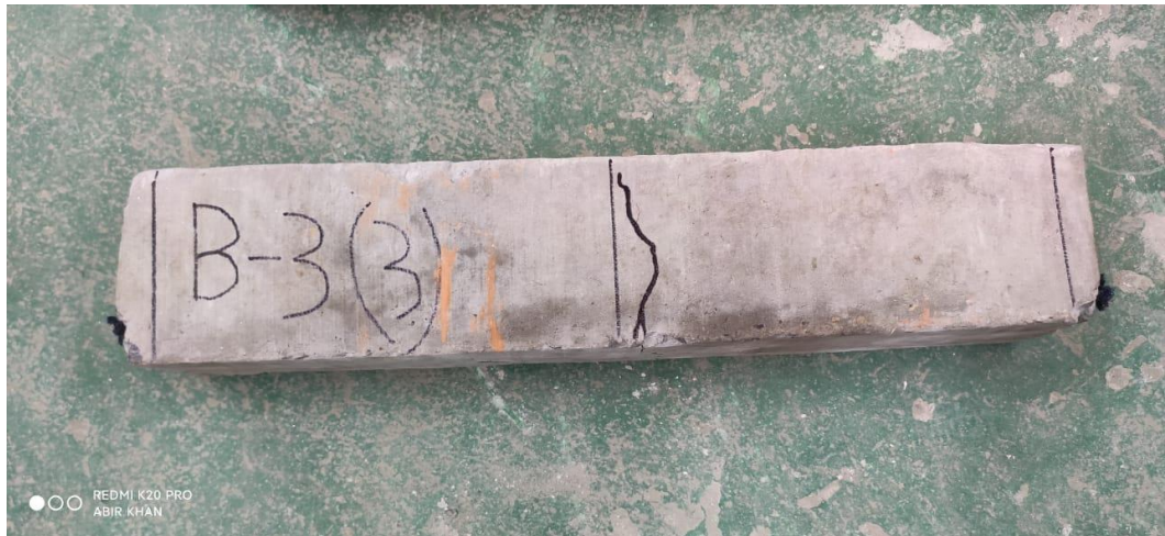
Figure 44: Failure pattern (for type 4 beam)
