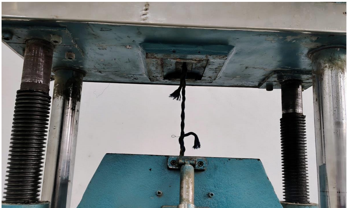
Figure 27: Tensile test for chemically submerged cotton fiber
