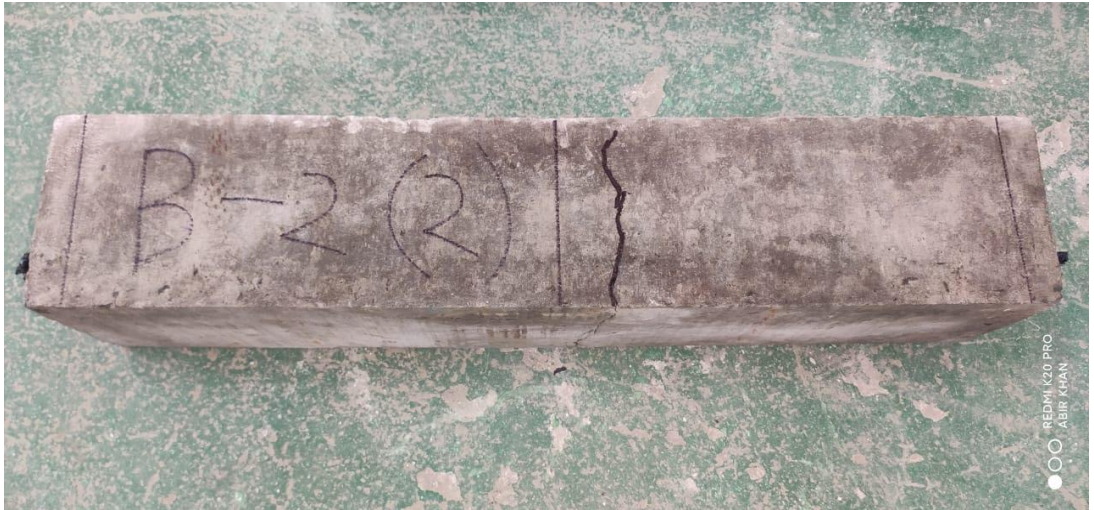
Figure 43: Failure pattern (for type 3 beam)
