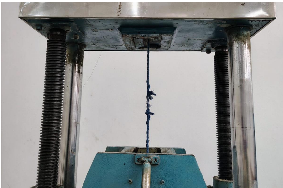
Figure 25: Tensile test of textile reinforcement
