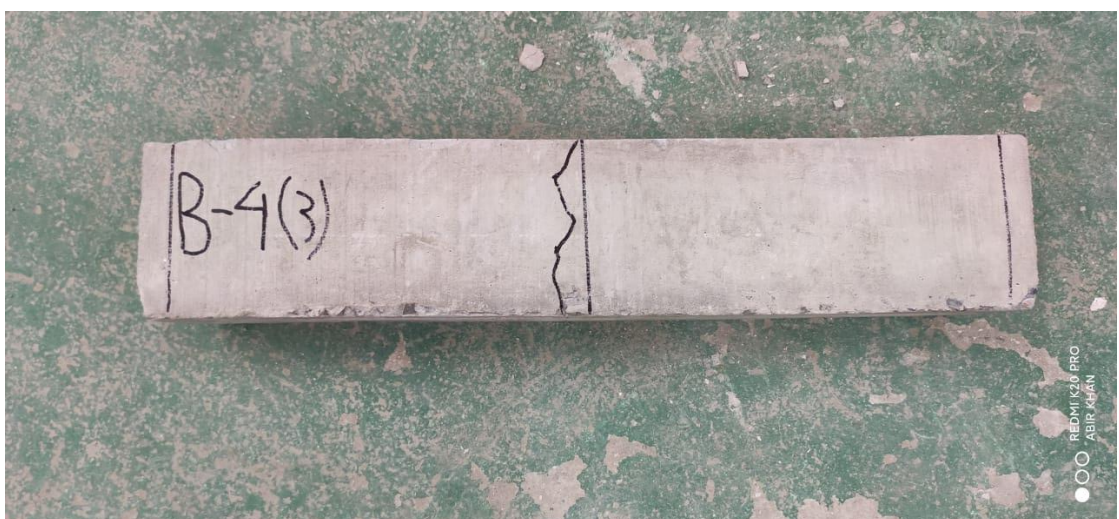
Figure 45: Failure pattern (for type 4 beam)
