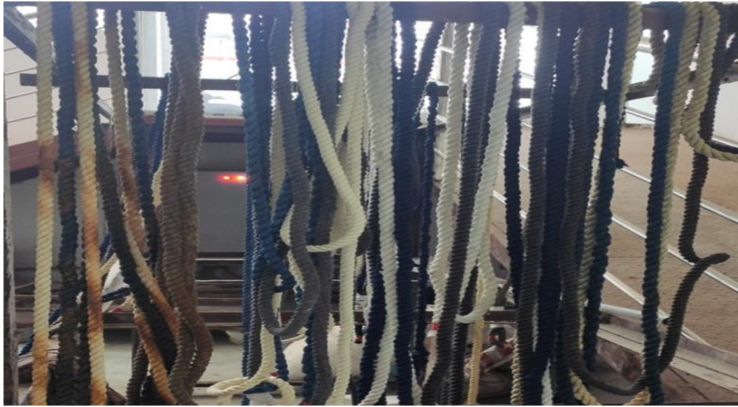
Figure 14: Chemical solution submerged cotton drying
