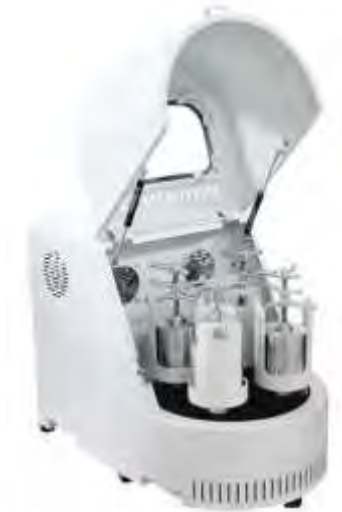
Figure 3.4 Planetary ball mill was used for rotor mixing.
