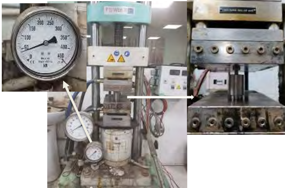
Figure 3.7 Cold Compression in a die using hydraulic press (P O/ Weber).
