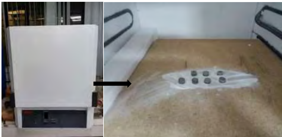
Figure 3.10 Sintering of samples using Lenton laboratory furnace (advanced wire chamber furnace)
