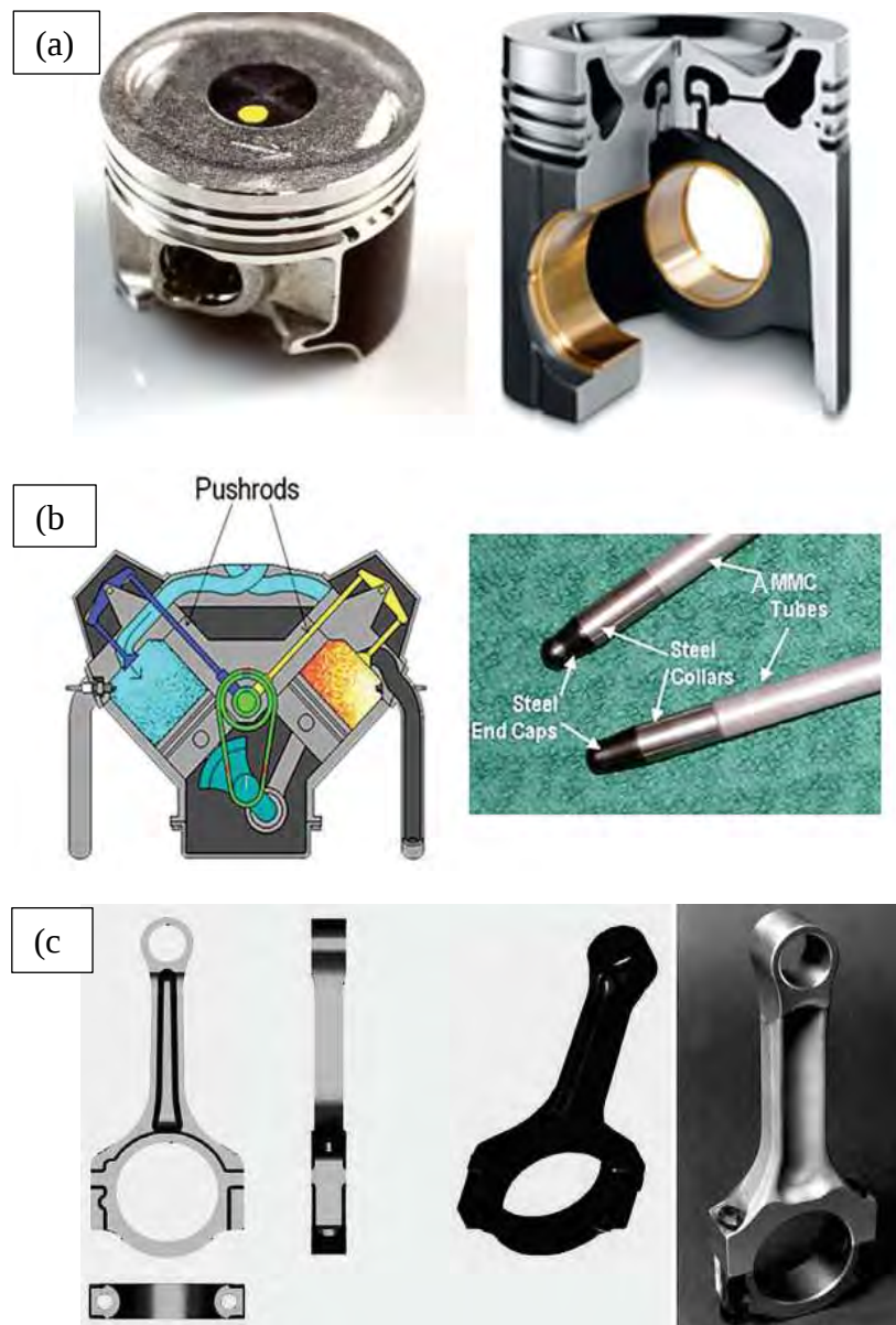
Figure 2.2 (a) Pistons made of AMMC , (b) Pushrods made of AMMC at engine , (c) Piston connecting rod [14].
