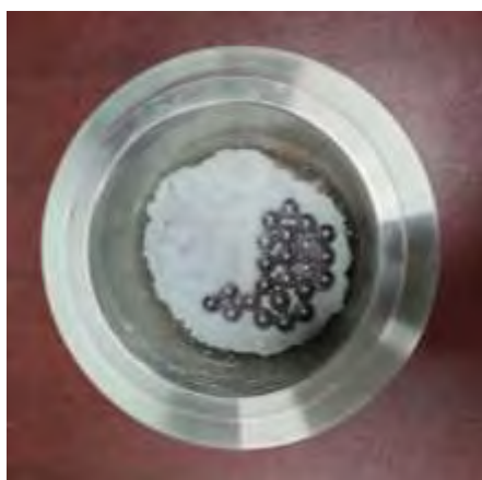
Figure 3.3 Well dispersed \text{TiO}_2 , \text{H}_3\text{BO}_3 within Al particles
