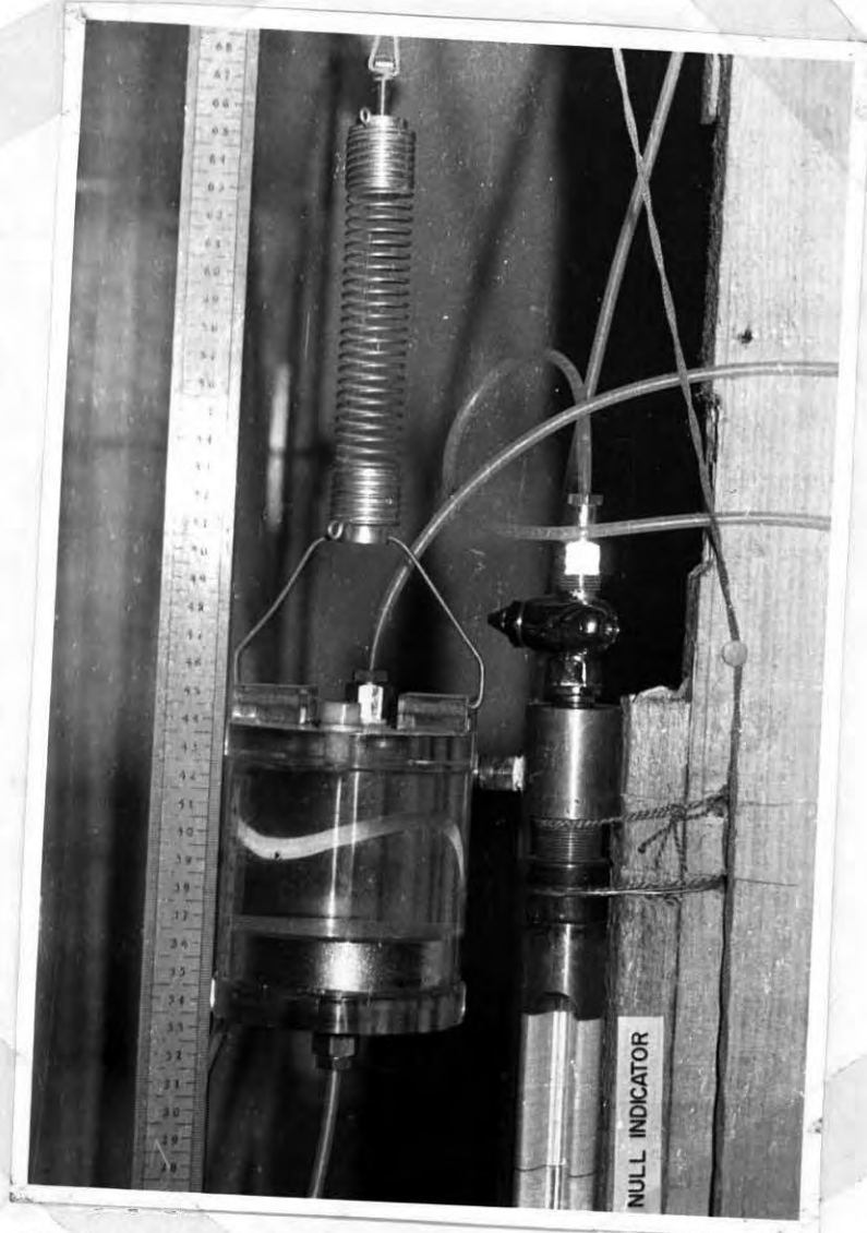
Plate 3.5 The Top Mercury Pot.
