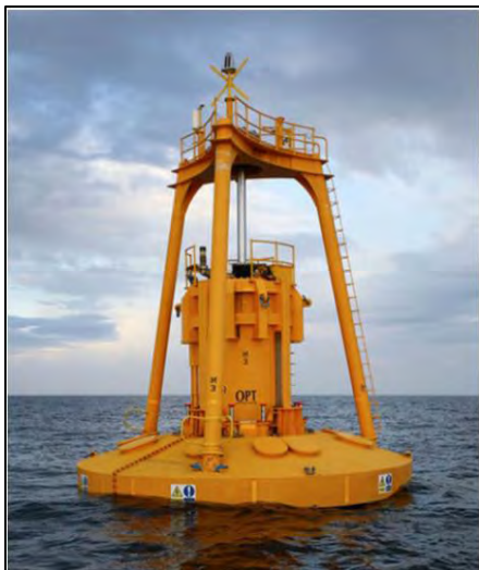
Figure 3.2 Floating point absorber (Source: Amir et. al, 2015)
