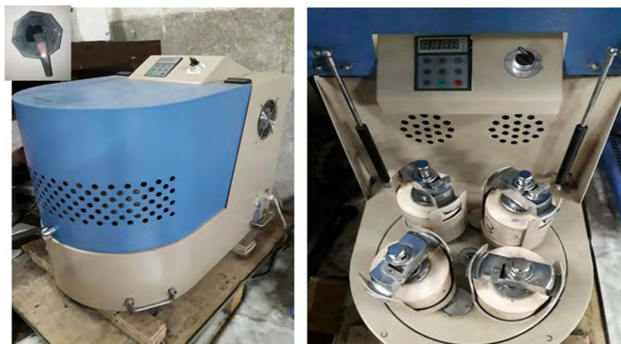
Fig. 3.4 Ball mill and its cross-section picture of MSK-SFM-1 benchtop planetary ball mill.
