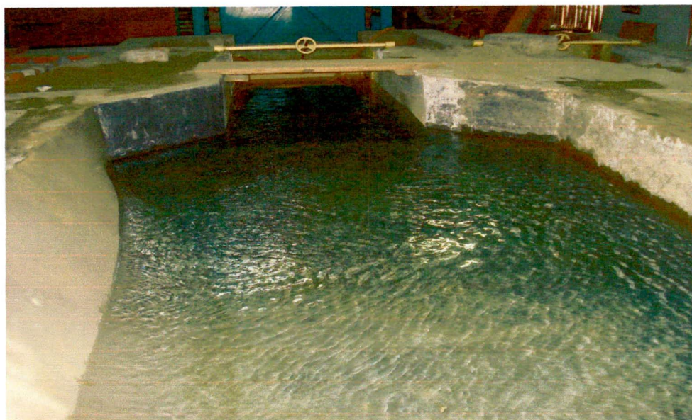
Figure 3.15 Test run in the Channel without apron
