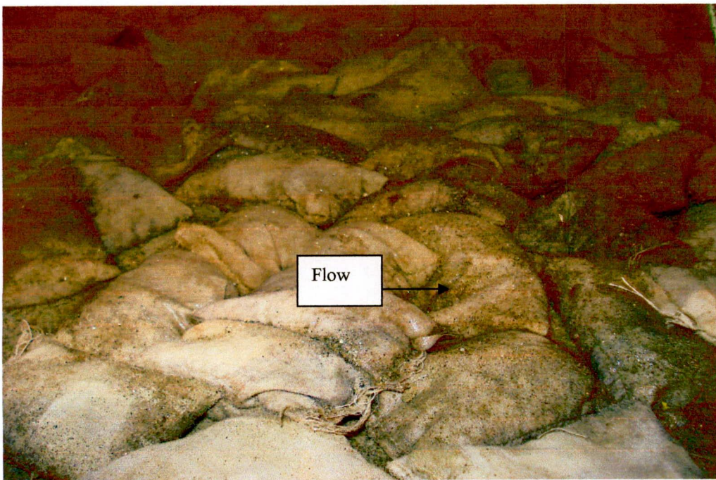
Figure 3.30 Flow over the Launching apron in 1:1.5 slope
