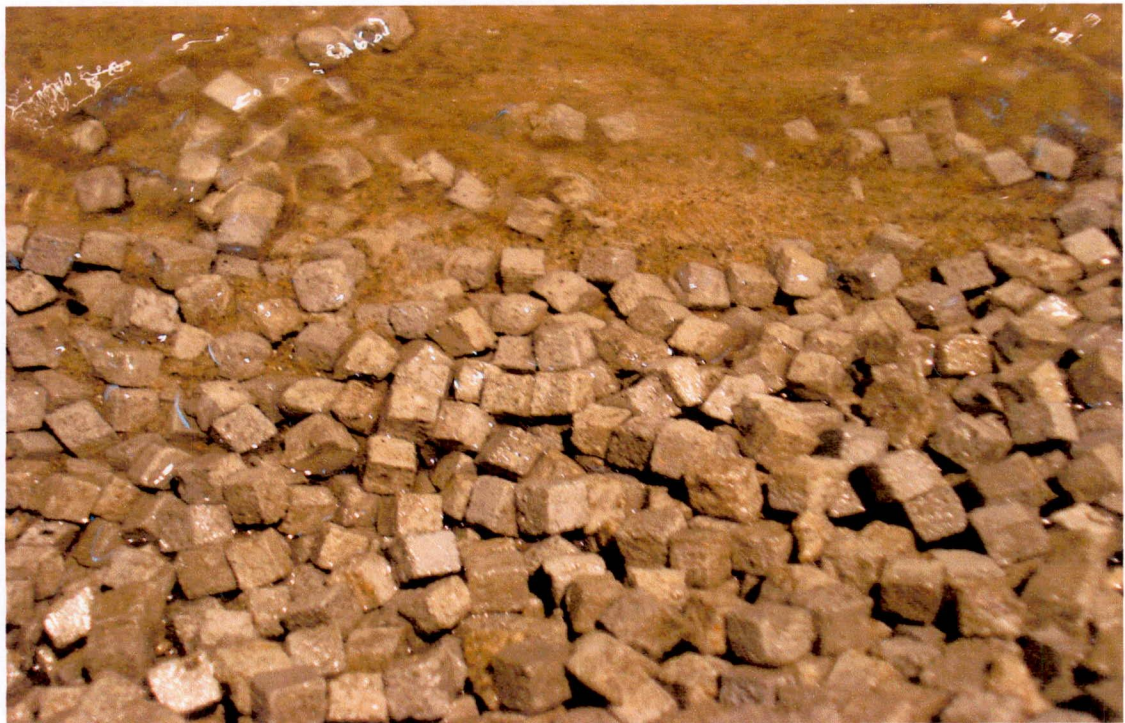
Figure 4.44 Photographs of launching of 4mm apron
