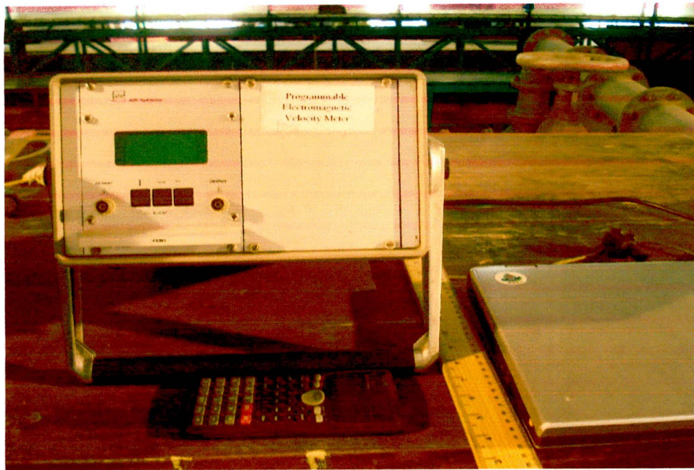
Figure 3.18 Control Unit of Electro Magnetic Velocity Meter (PEMS)
