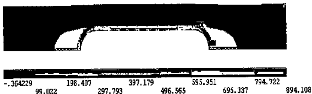
Figure 5.22: Plot of the first principal stresses for the RVE (short CNT) with 1.2 nm of CNT wall thickness under axial stretch ( \Delta L = 1 nm).
