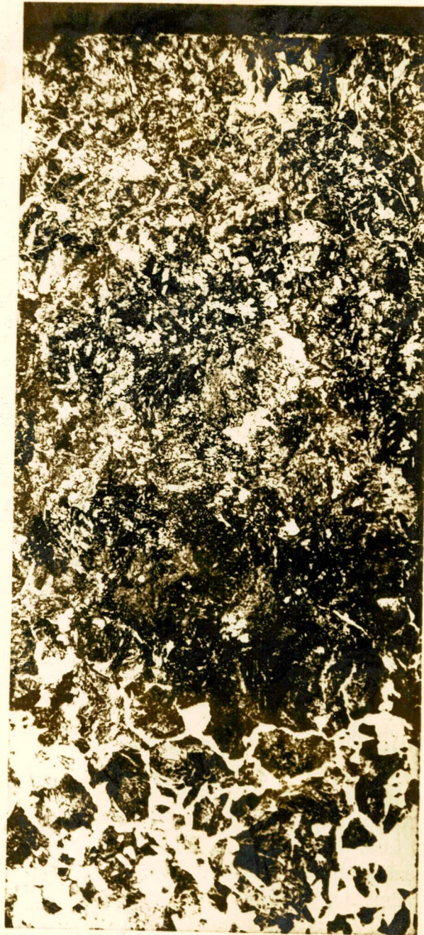
FIG. 8 Carburized Steel (100×) High-Carbon Case at Top Low-Carbon Core at Bottom 8
