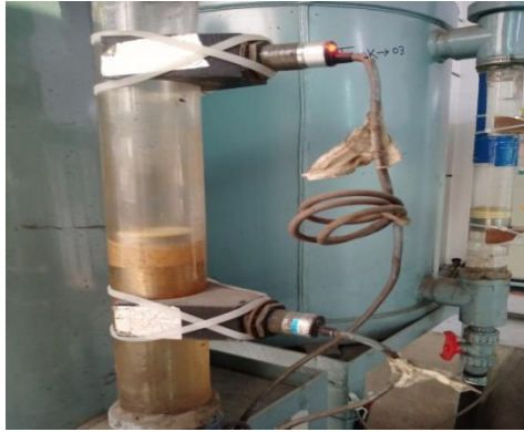
Figure 12; Capacitive Type Proximity Sensor.
