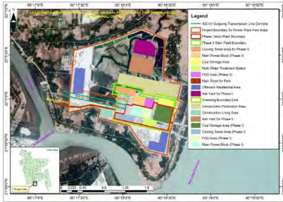
Figure 3.2: Google Image Showing the Payra Thermal Power Plant Footprint Area (EQMS, 2018)
