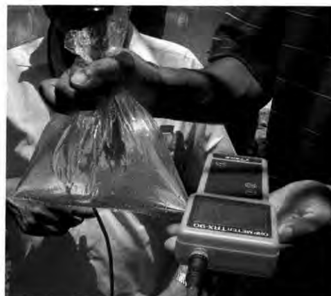
Figure 3.7: Measuring of Eh by inserting probe inside the bag
