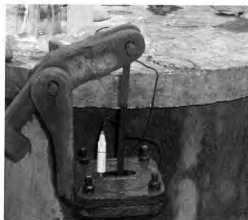
Figure 3.8: Measuring of Eh by inserting probe inside the top opening
