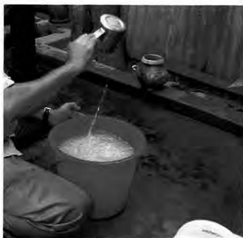
Figure 3.4: Mixing of bleaching powder with DW water
