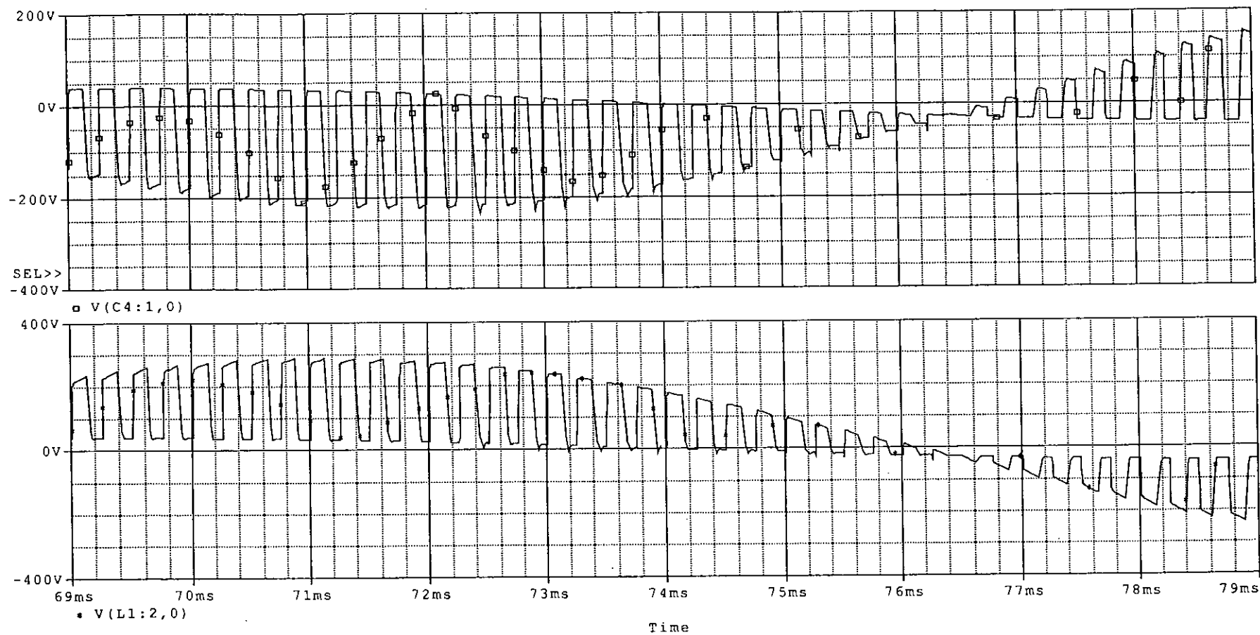
Figure-36. Voltage waveform across switches with snubber circuit.
