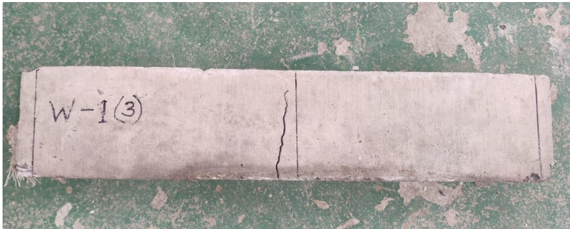
Figure 4-16: Failure Pattern for NRC-1(3-12mm)
