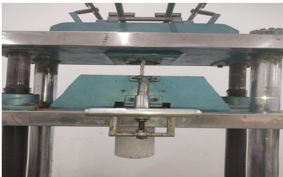
Figure 3-17: Pull-Out Test for UTM
