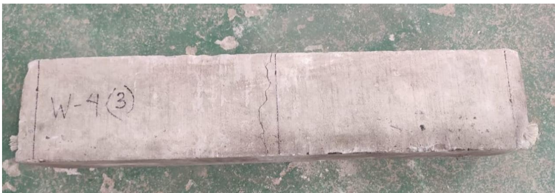
Figure 4-17: Failure Pattern for NRC-2(3-12mm)
