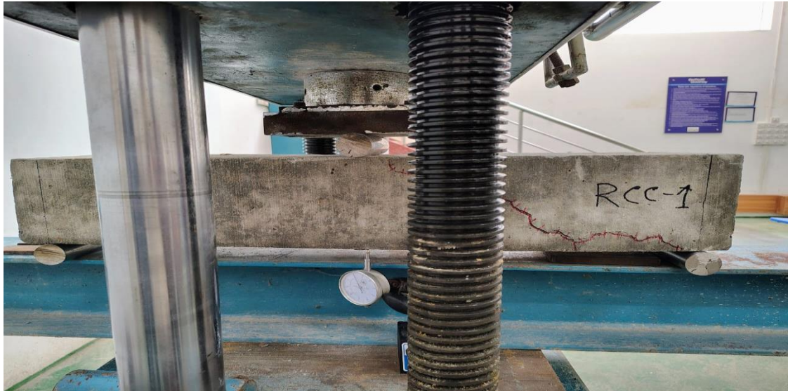
Figure 4-12: Failure Pattern for Reinforcement Concrete-1
