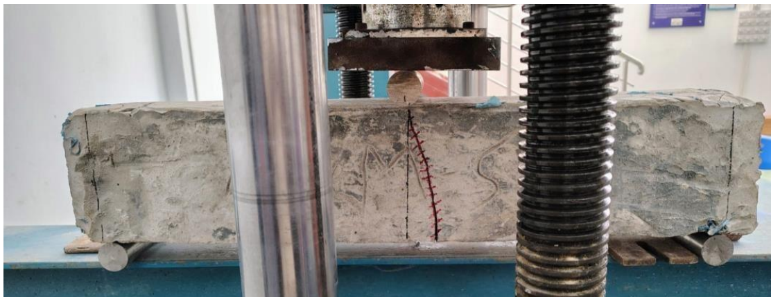
Figure 4-10: Failure Pattern for Pure Concrete-1
