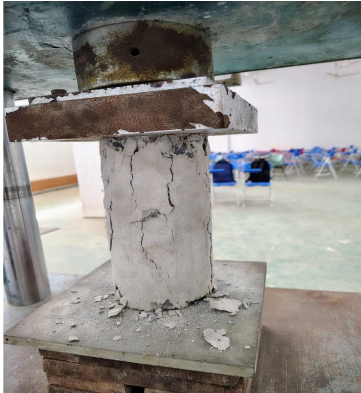
Figure 3-10: Compressive Strength Test for Slender
