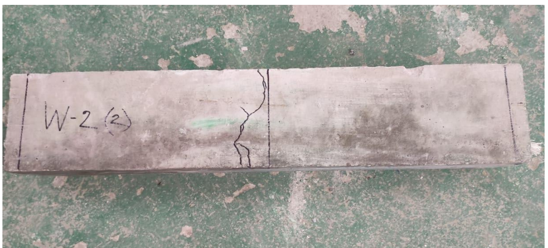
Figure 4-14: Failure Pattern for NRC-1(2-12mm)
