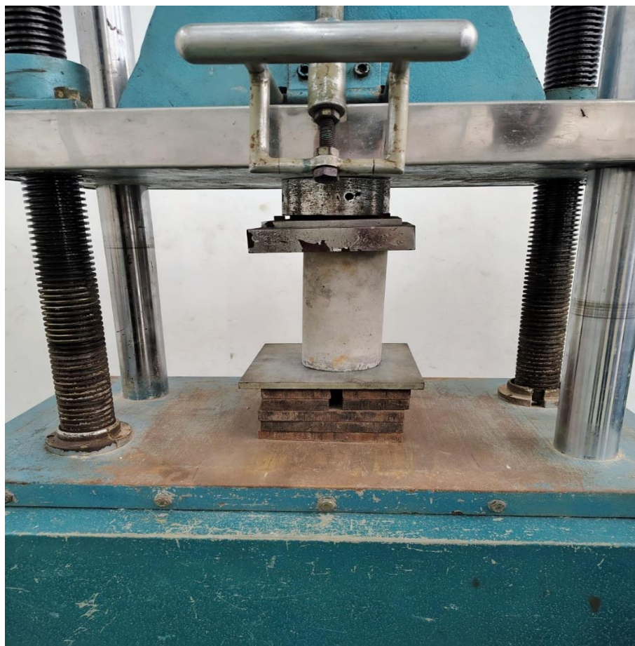
Figure 3-9: Compressive Strength Test for Slender
