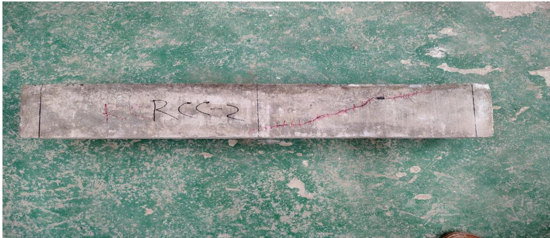
Figure 4-13: Failure Pattern for Reinforcement Concrete-2
