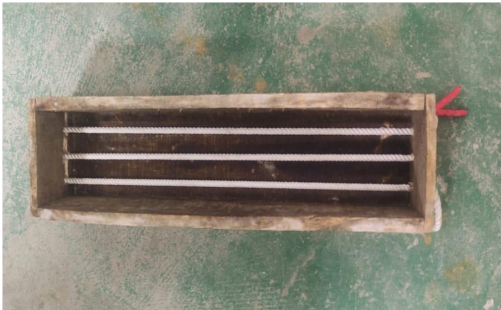
Figure 3-21: 3-12mm diameter bar Nylon Fibers
