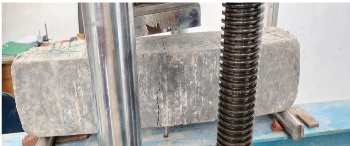
Figure 4-11: Failure Pattern for Pure Concrete-2
