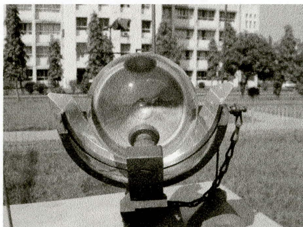
Figure 3-7: Sunshine Recorder at BMD, Dhaka
