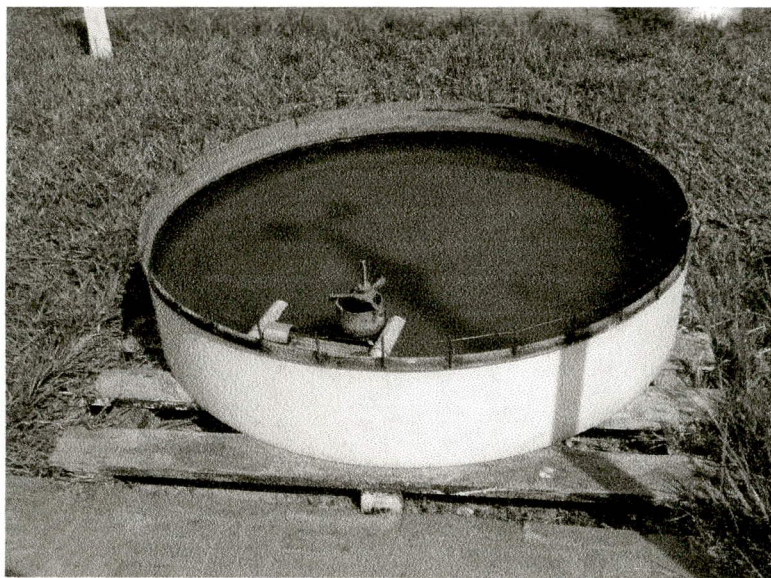
Figure 3-1: Evaporation Pan at BMD, Dhaka
