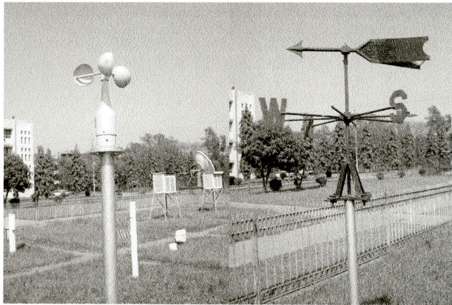
Figure 3-4: Cup Anemometer (Left) and Wind Direction Measurement (Right) at BMD, Dhaka
