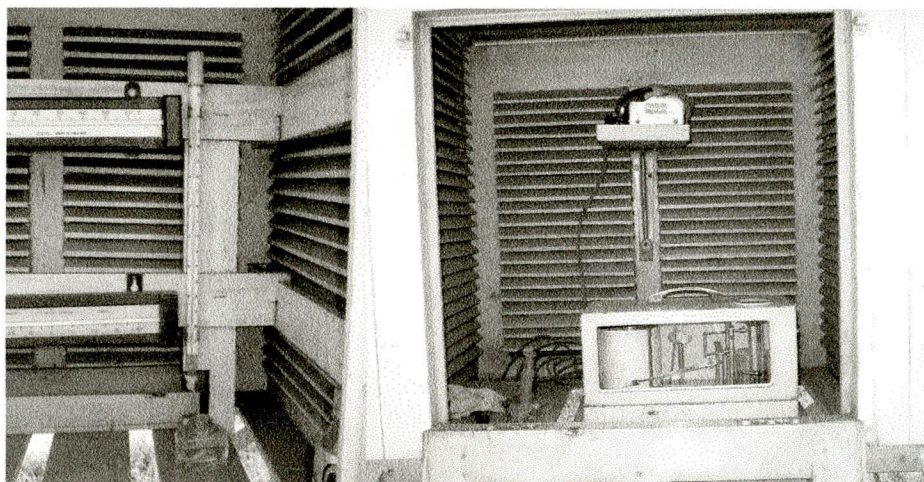
Figure 3-6: Wet Bulb Thermometer (Left) and Auto Humidity Recorder (Right)
