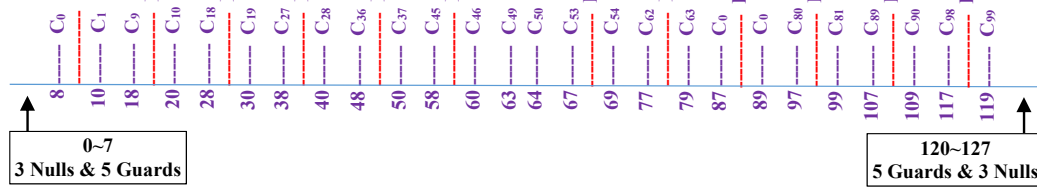
Fig. 1.4: Position of the MB-OFDM UWB Subcarriers in 128 Point IFFT [17,21]
