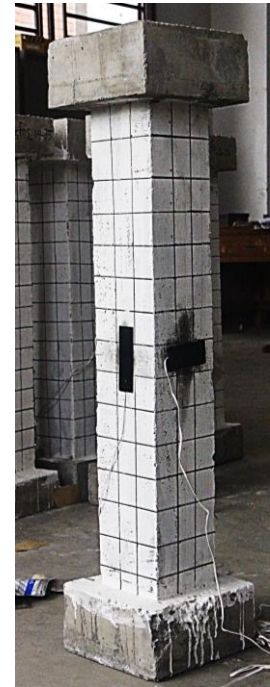
(b) Installation of Concrete Strain Gauge on Column Surface
