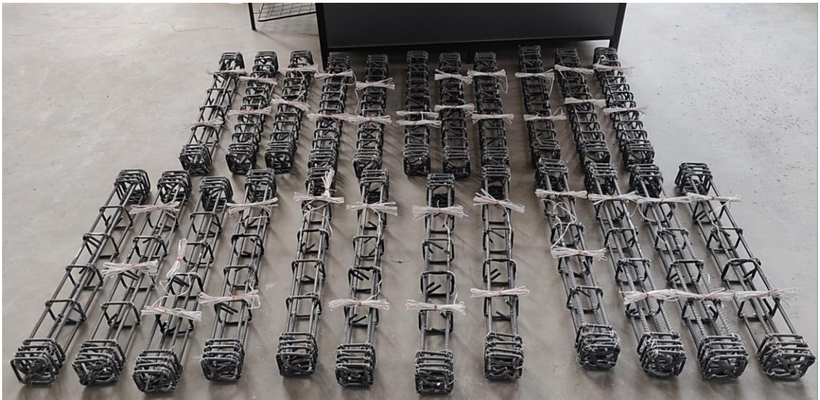
(c) All Columns After Installation of Strain Gauges
