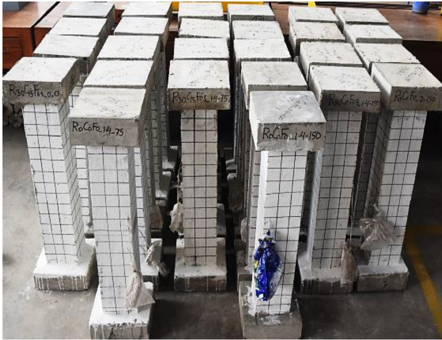
(a) Whitewashed and Gridded the Columns' Surfaces
