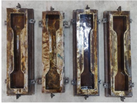
(c) Preparation of Dog Bone Molds
