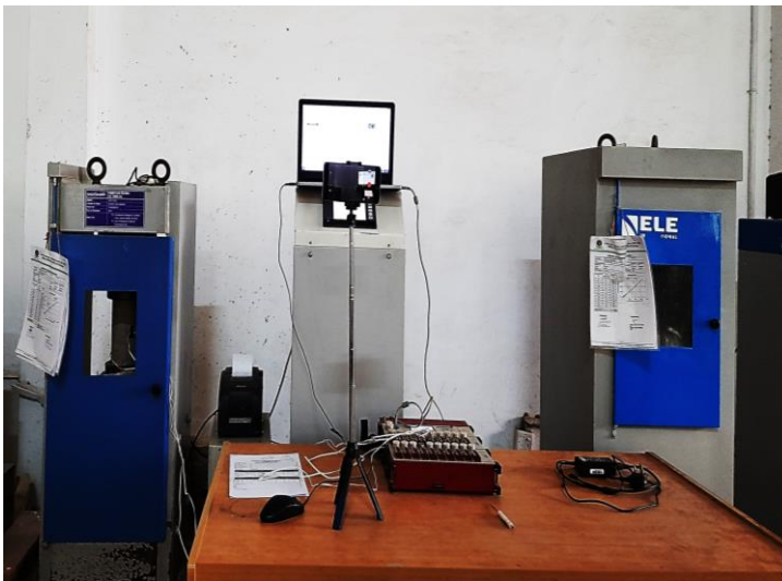
(a) Compressive Strength Test of Concrete Cylinders
