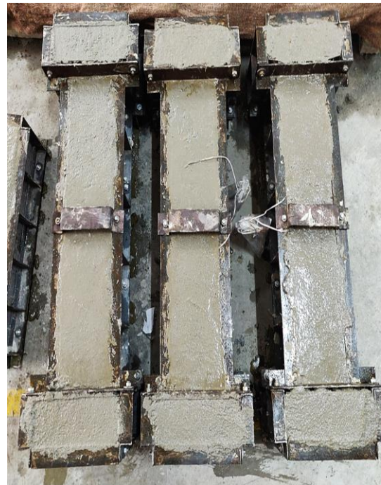
(b) Casting of Columns Specimens
