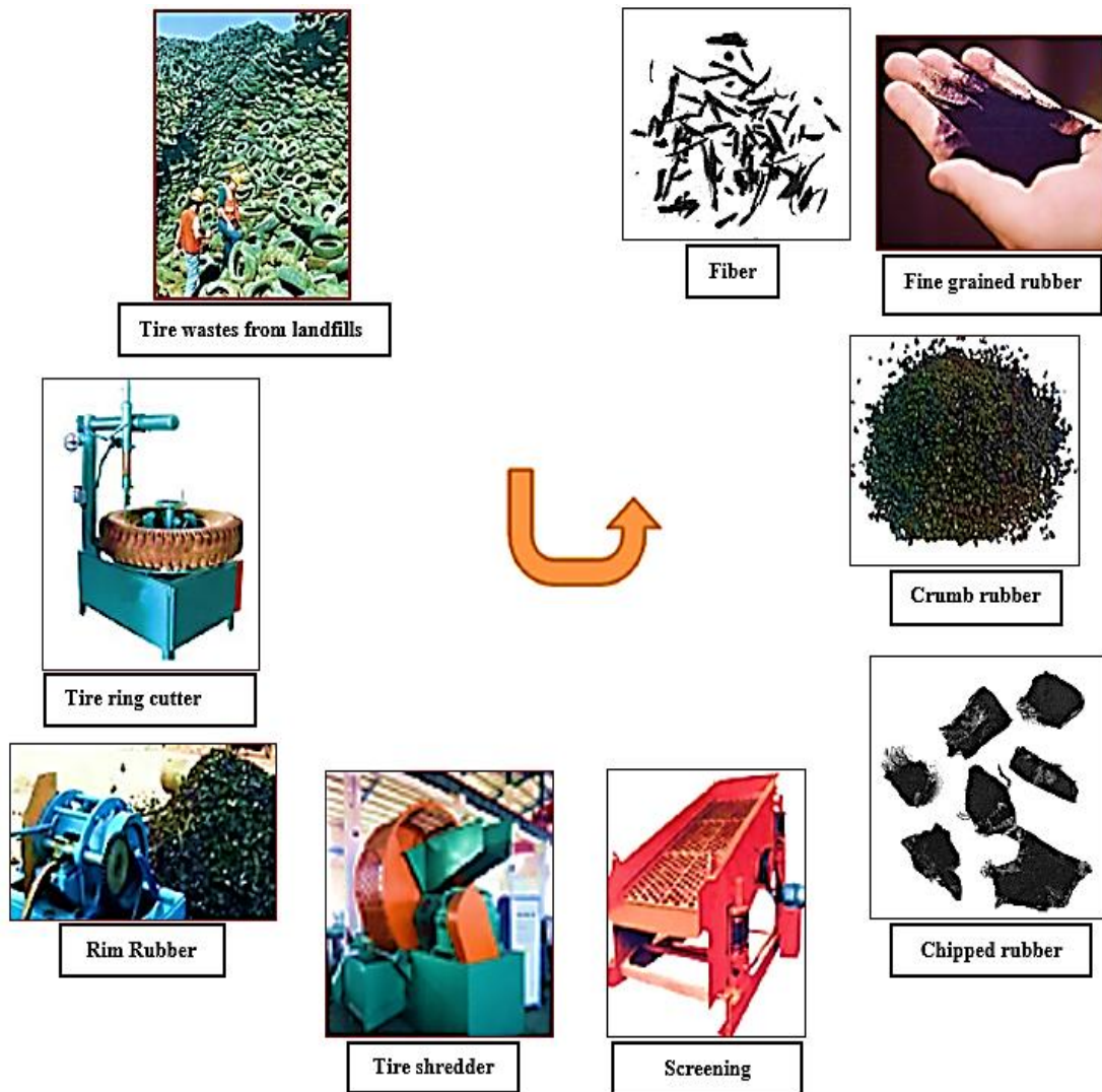
Figure 2.2 Stage-wise process of tire-shredding (modified images from sources [40, 51-53]).
