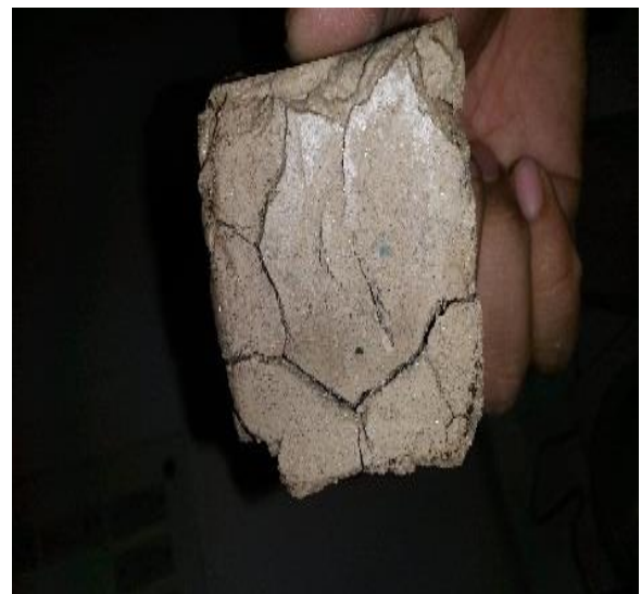
(l) Ignoring excessively cracked samples
