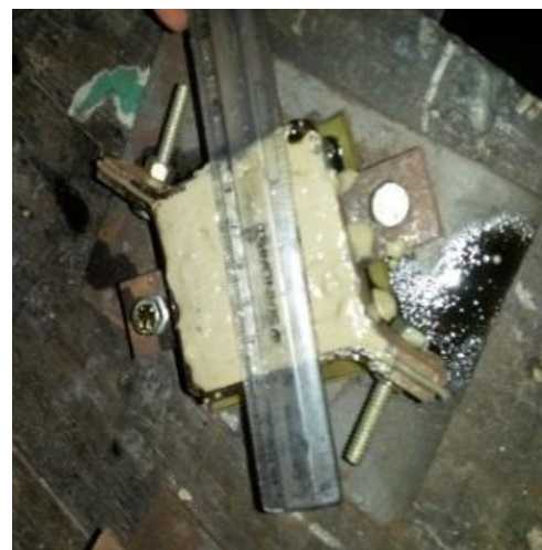
(f) Ensuring smoothness of top surface
