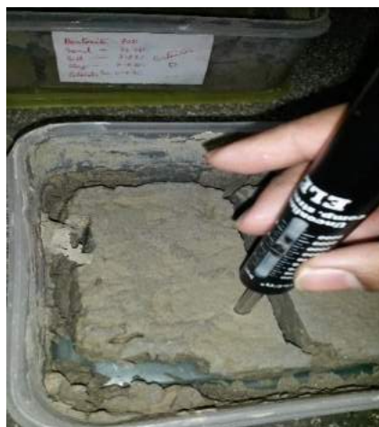
Figure 3.40: Reading on miniature pitch by penetrometer
