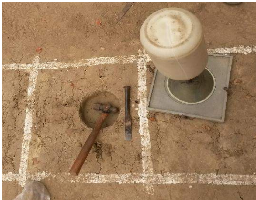
Figure 3.52: Field density test of bullis
