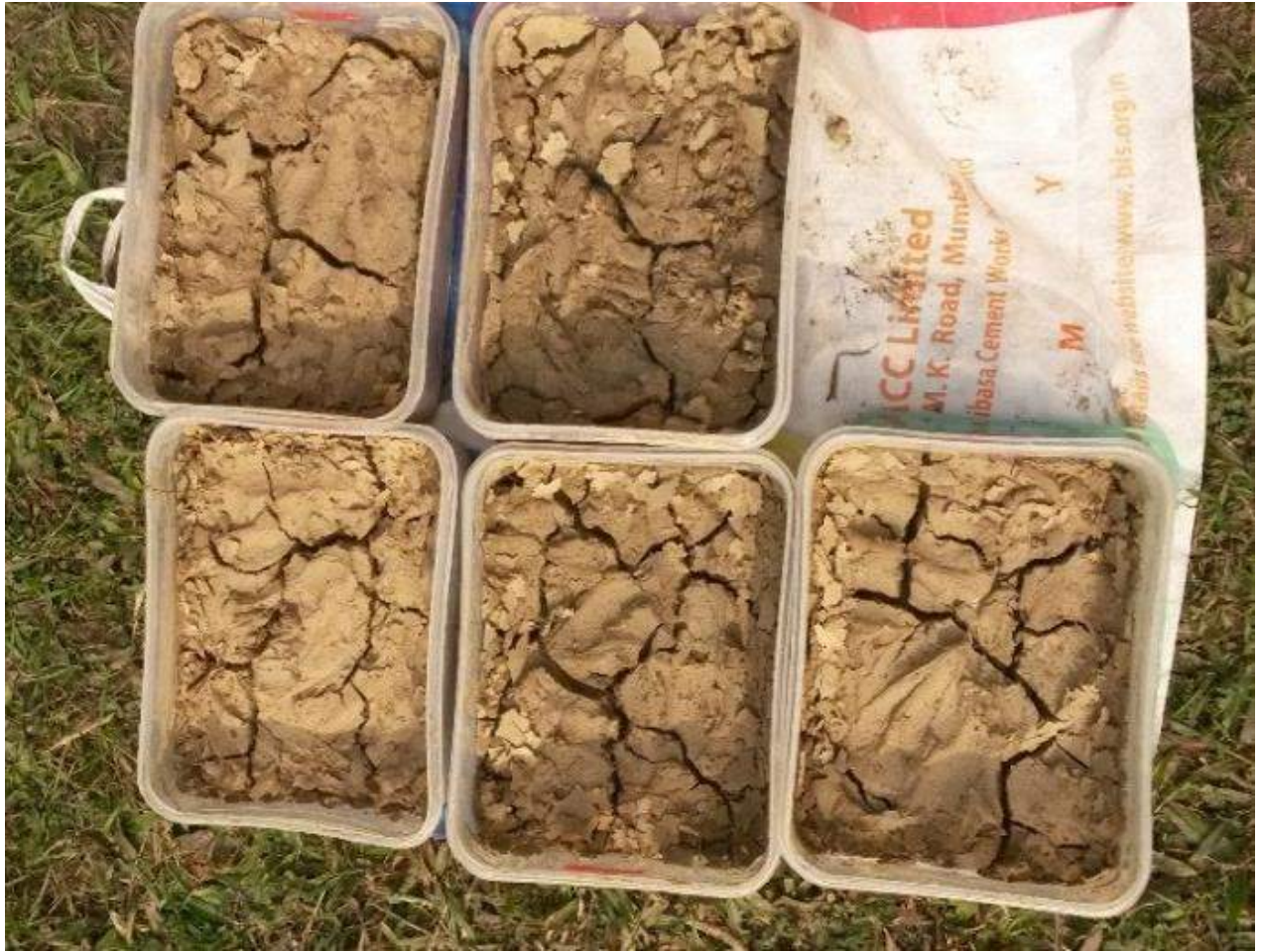
Figure 3.17: Typical crack pattern of different composition of bulli
