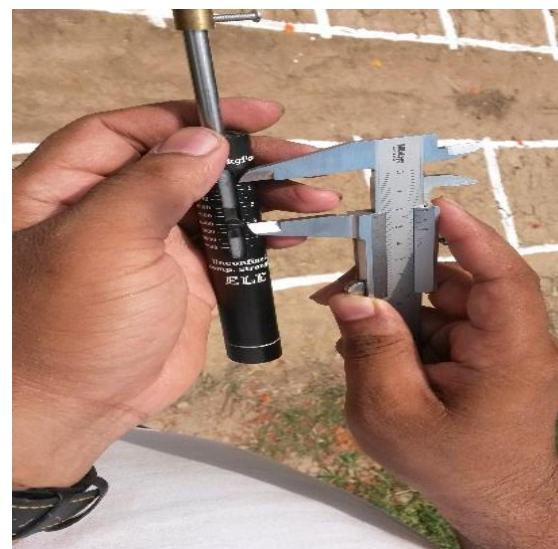
(b): Measuring the deflection of indicator
