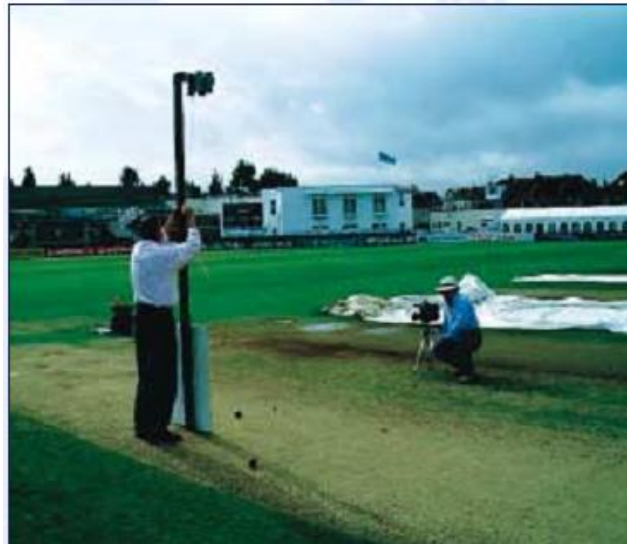
Figure 2.7: Three meter ball drop test
