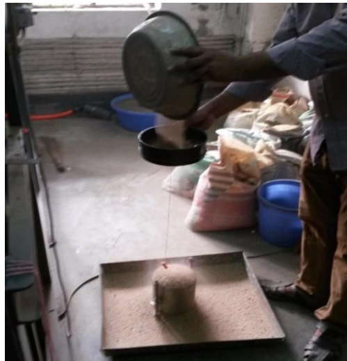
Figure 3.5: Arrangement of maximum self-compaction height test
