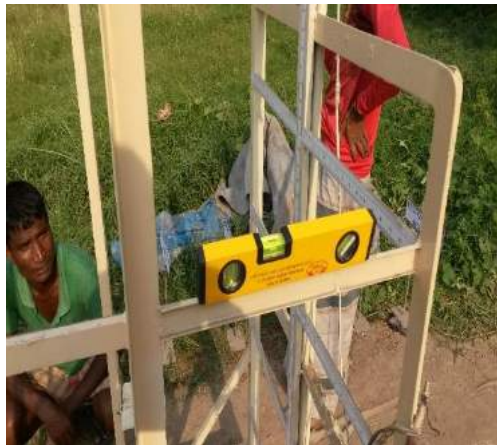
Figure 3.44: Leveling the bounce meter by water level
