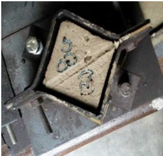
(i) Collection of cube samples after 7 days
