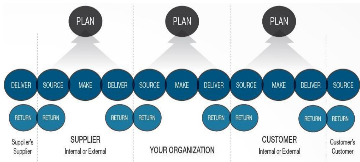
Figure 3.1: Interrelation of five key processes of SCOR (Source: www.supply-chain.org , 2013)
