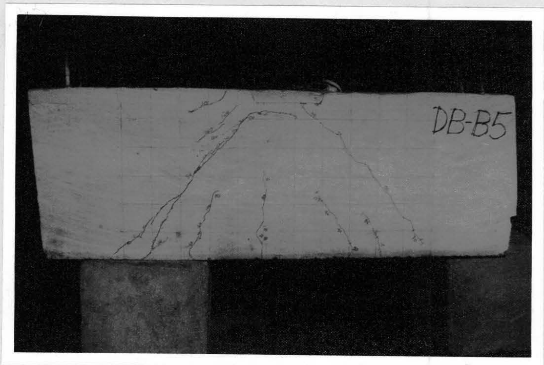
Fig. 5.48 Observed mode of failure and the crack pattern of Beam DB-B5
