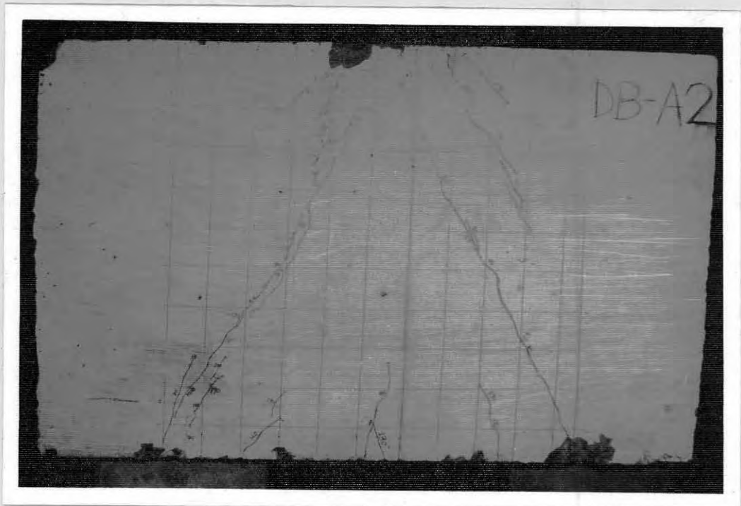
Fig. 5.40 Observed mode of failure and the crack pattern of Beam DB-A2
