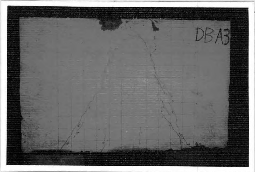
Fig. 5.41 Observed mode of failure and the crack pattern of Beam DB-A3
