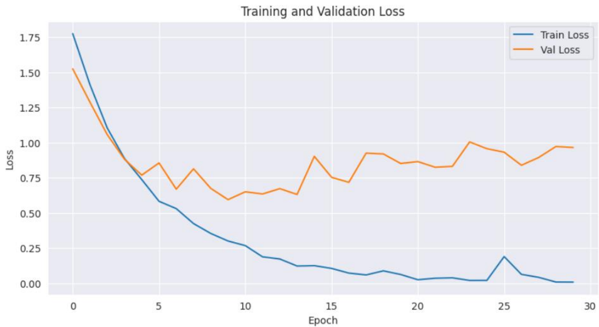
Figure 5.3.5 Model accuracy and loss curve of CNN
