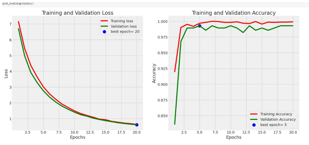
Figure 5.3.4: Model accuracy and loss curve of Xception
