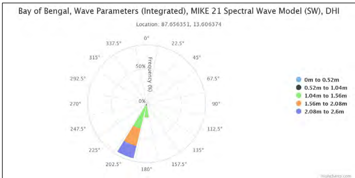
Figure 3 13: Wave rose for October 2007 for calibration (Latitude: 13°60', Longitude: 87°65')
