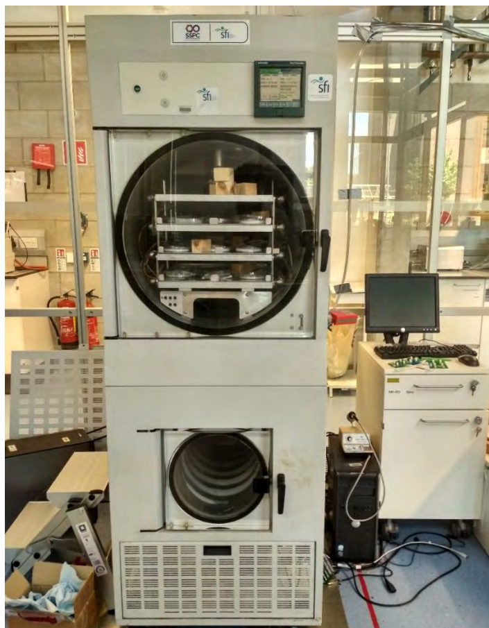
Figure 4.4: The dialyzed sample was freeze-dried in Severn Freeze-Dryer.
