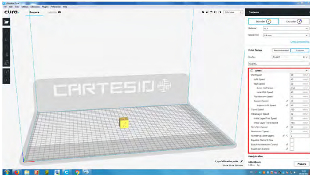
Figure 3.11: Cartesio FDM 3D printer's settings for 'printing speed'.
