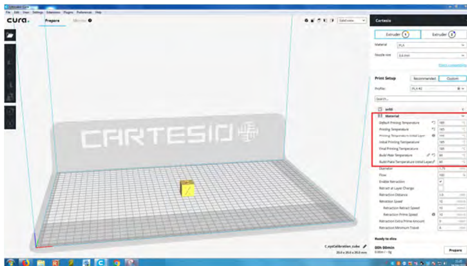
Figure 3.12: Cartesio FDM 3D printer's settings for temperature control.
