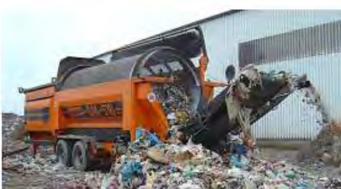
Photograph-7.2: Trommel Drum Screen Proposed for Physical Separations and Mixing Organic Waste with Stabilizers, adapted from [104]
