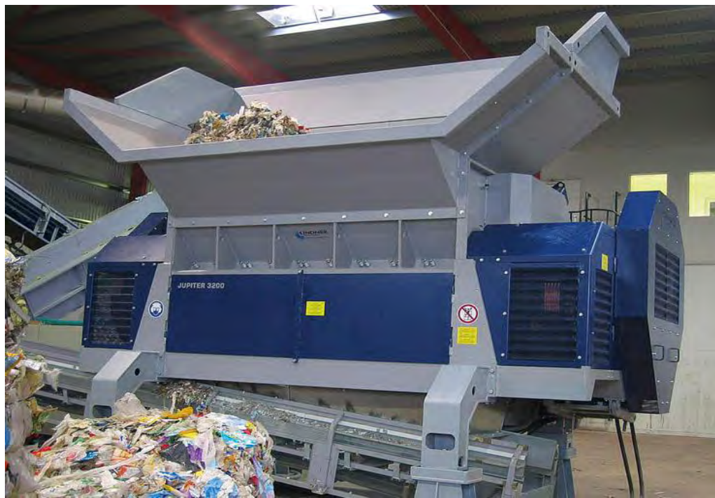
Photograph-7.1: Primary Shredder Proposed for Size Reduction of Organic Waste, adapted from [102]
