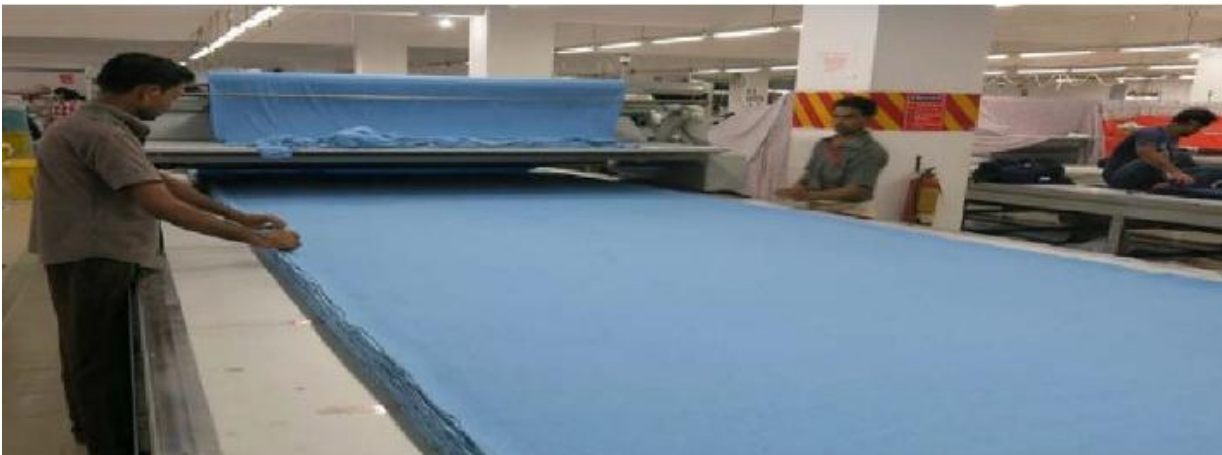
Fig: Automatic Spreading
