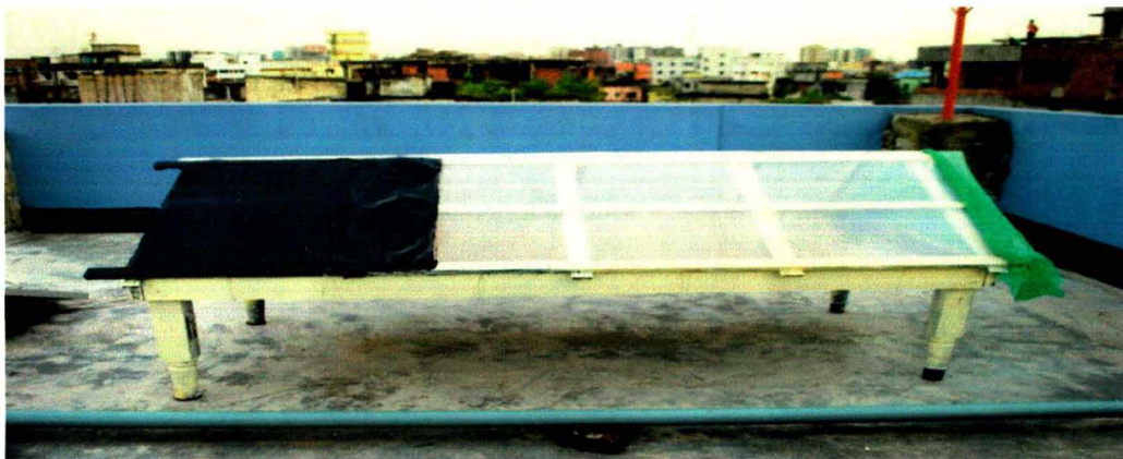
Plate 8A. Showing external and partial of the low cost solar tunnel dryer constructed at the Fish Tec. Laboratory for drying and dehydration of the experimental fishes using locally available raw materials.
