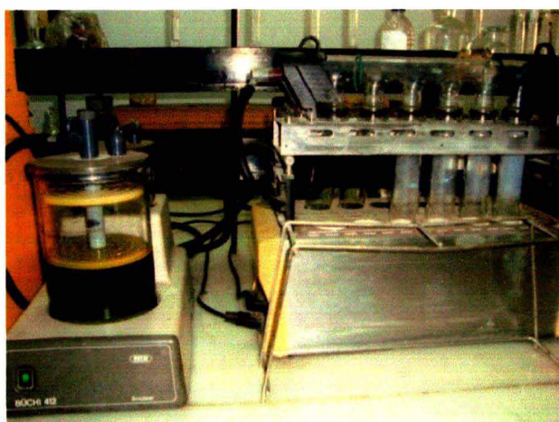
Plate 16. Showing different steps determination of protein content content of the fish samples by micro-kjeldhal method in the laboratory.
