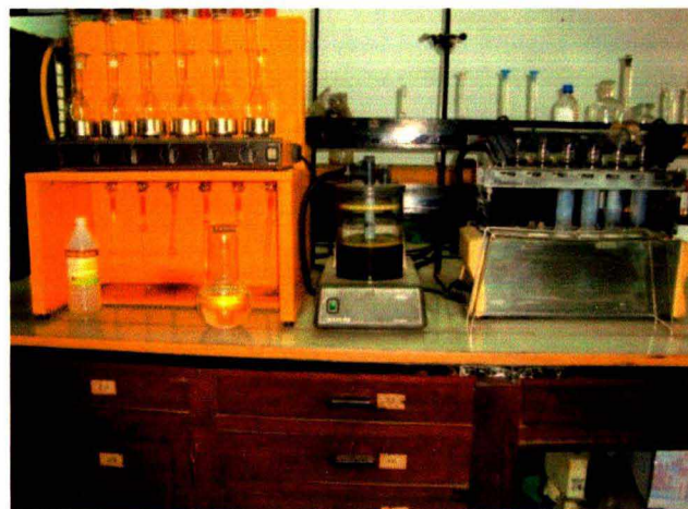
Plate 16. Showing different steps determination of protein content content of the fish samples by micro-kjeldhal method in the laboratory.
