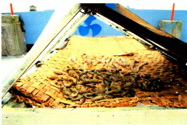
Plate 9. Showing the solar tunnel dryer during drying and dehydration of the experimental fishes ( Pampus chinensis , Harpodon nehereus ) and P. monodon at the experimental at label.
