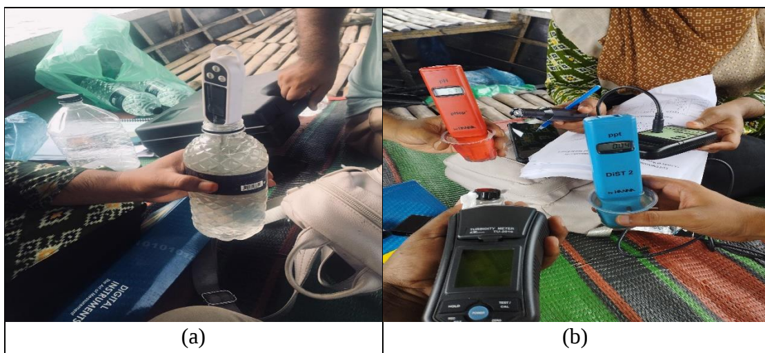
Fig. 3.4 On spot physiochemical parameters test (a) Temperature Test, (b) Turbidity, pH, DO, EC test
