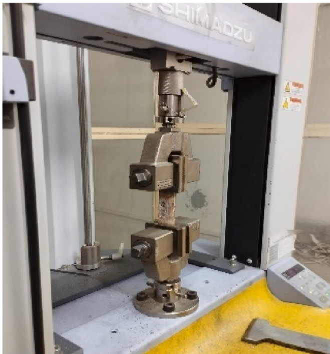
Fig. 6. Universal Testing Machine with the tensile test setup.
