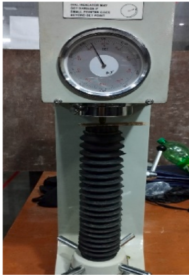
Fig. 9. Rockwell hardness test setup.
