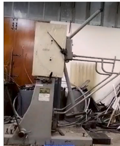
Fig. 8. Charpy impact test setup.
