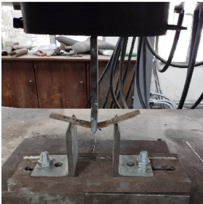
Fig. 7. Universal Testing Machine with the flexural test setup.
