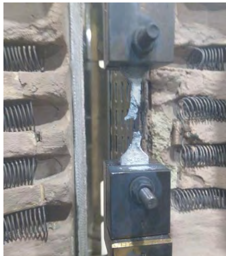
Figure 4.11: Oxide formation of Mg-1Ca-4Sn alloy during tensile test at 450°C and strain rate 1 \times 10^{-4} \text{ s}^{-1}
