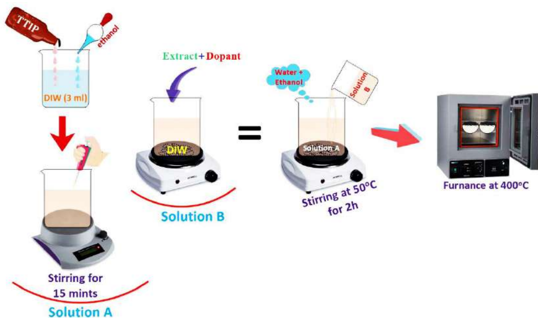
Figure 3.1: Overview of the TiO_2 green synthesis procedure.
