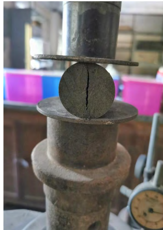
(b) 20% SDA – Brittle Failure
