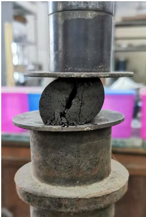
(a) 0% SDA – Ductile Failure
