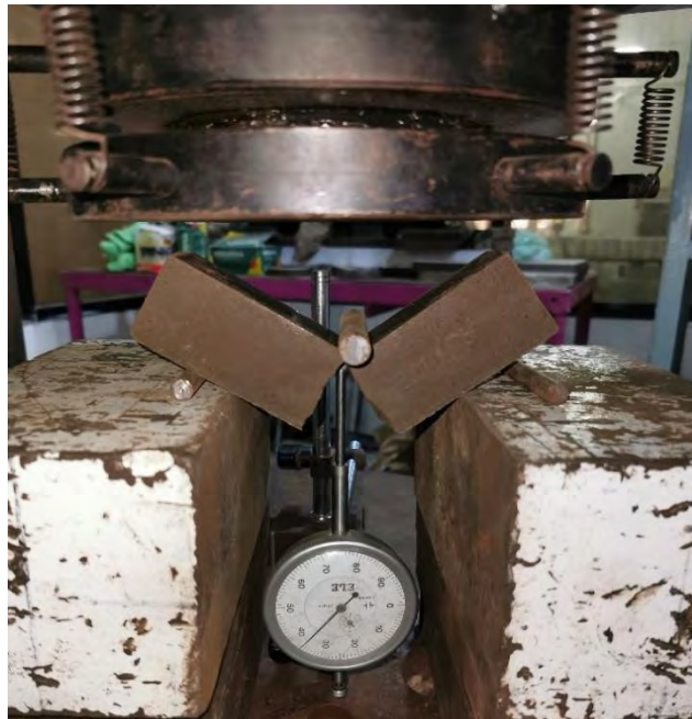
Figure 4.14: Typical failure mode in flexure strength test
