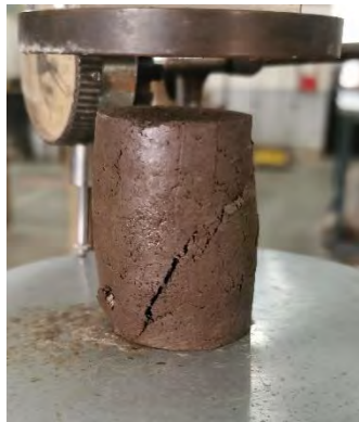
(c) Bulging, Shear Failure
