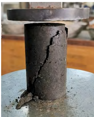
(f) Shear Failure
