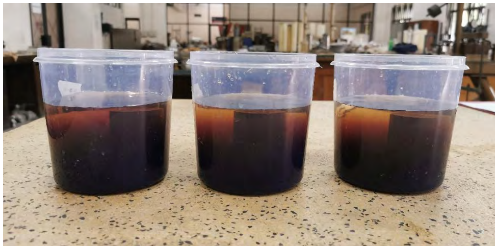
Figure 3.10: Samples after 24 hour oven drying at 105°C
