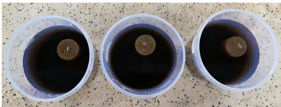
Figure 3.11: Samples after 24 hour water submersion (a) elevation and (b) plan view
