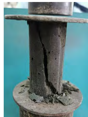
(g) Shear, Vertical Crack
