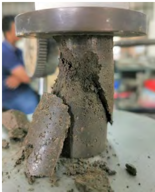
(b) Shear Failure
