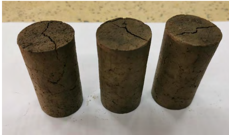
Figure 3.10: Samples after 24 hour oven drying at 105°C
