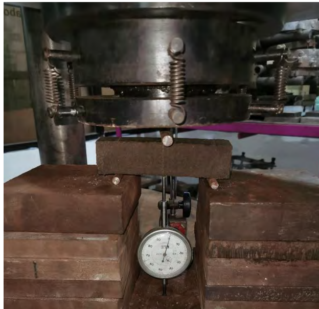
Figure 3.9: Test setup for center-point bending test to determine flexural strength
