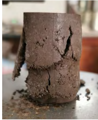
(a) Bulging Failure
