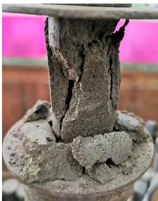
(e) Shear, Vertical Crack
