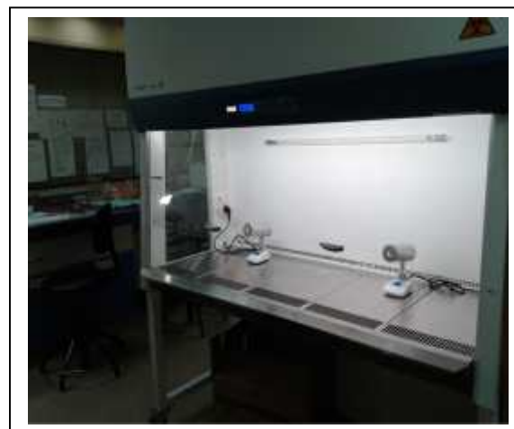
Fig.-8.6: Biosafety Cabinet for microbial culture
