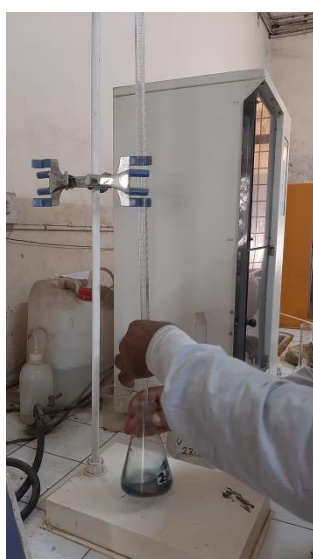
Plate 15. Total nitrogen determination (A: digestion; B: Distillation and C: titration)
