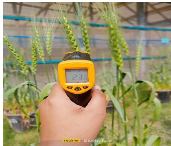
Plate 7: Photos showing measurement of temperature of flag leaf using infra-red thermometer.
