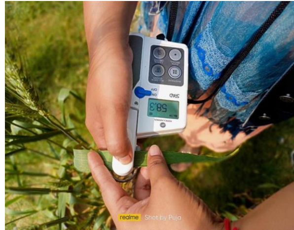
Plate 6: Photos showing measurement of SPAD value of flag leaf using SPAD meter.
