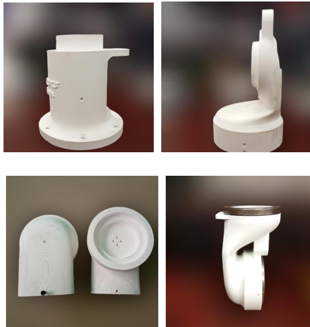
Figure 35 : a) Base, b) Shoulder, c) Elbow, d) Wrist
