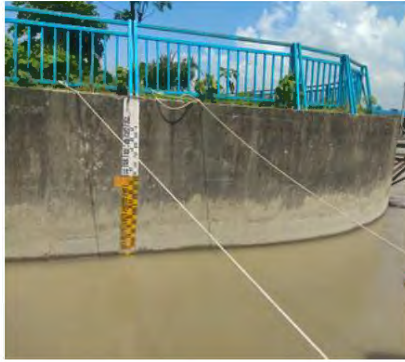
4. a) Water level measurement at Dalia point
