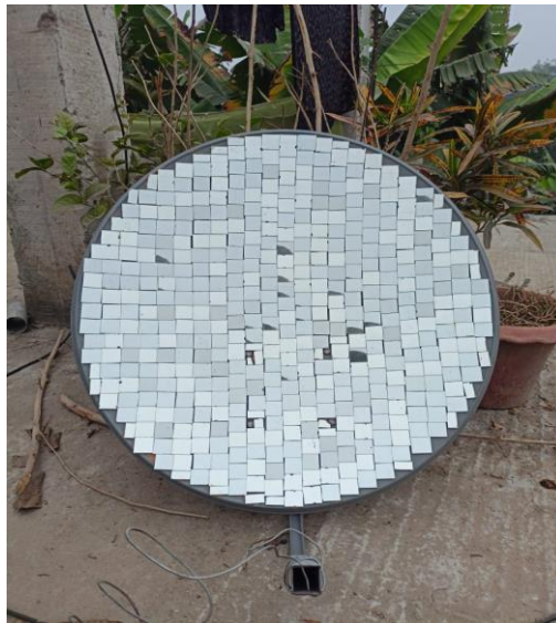
Figure 4.1: Focus test on parabolic dis
