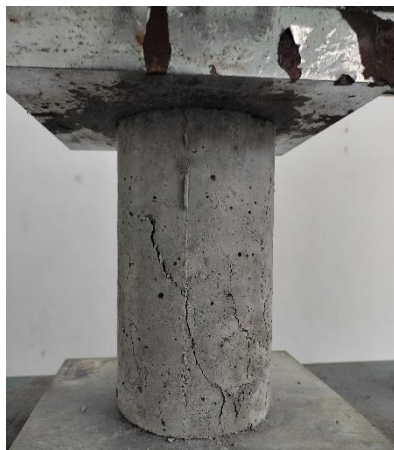
Fig. 3-13 Compressive strength test
