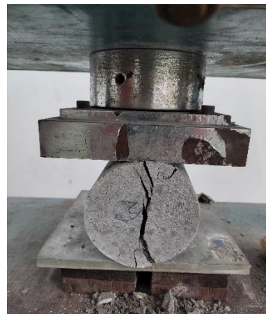
Fig. 3-14 Tensile strength test
