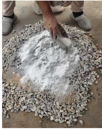
Fig. 3-10 Mixing eggshells with sand, cement, stone
