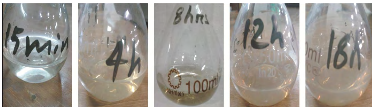
Fig. 3.24 Optical image of ammoniacal silver solutions after reacting with dopamine added paper with different time intervals.
