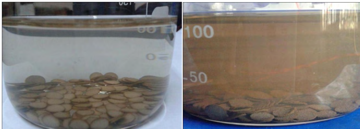
Fig. 3.15 Optical image of the deposition of AgNPs onto dopamine added paper surface (left one) deposition time one minute (right one) deposition time 12 hours.
