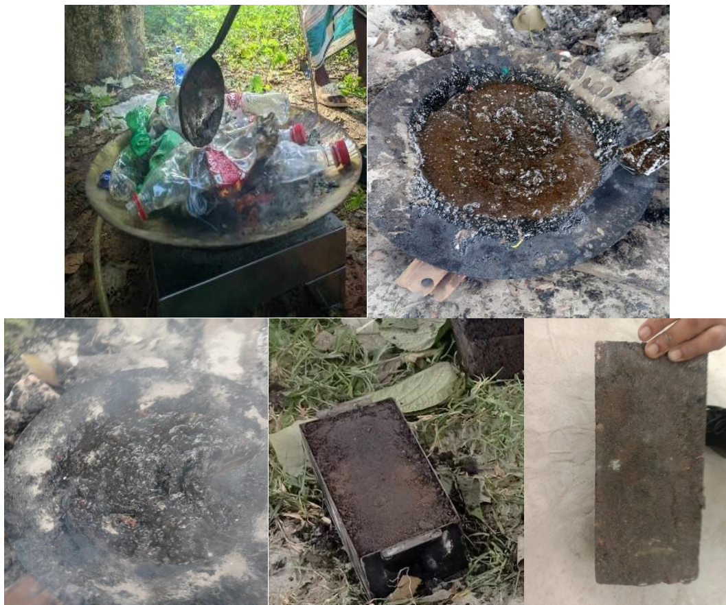
Figure 3-1 : producing bricks out of plastic bottle
