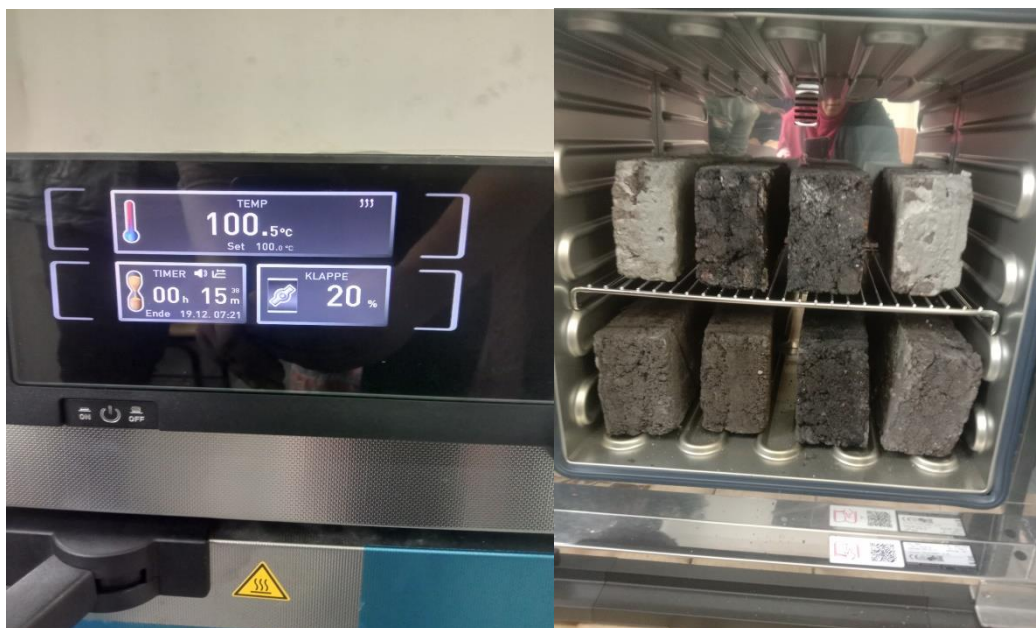
Figure 3-2 Temperature measure& dry process
