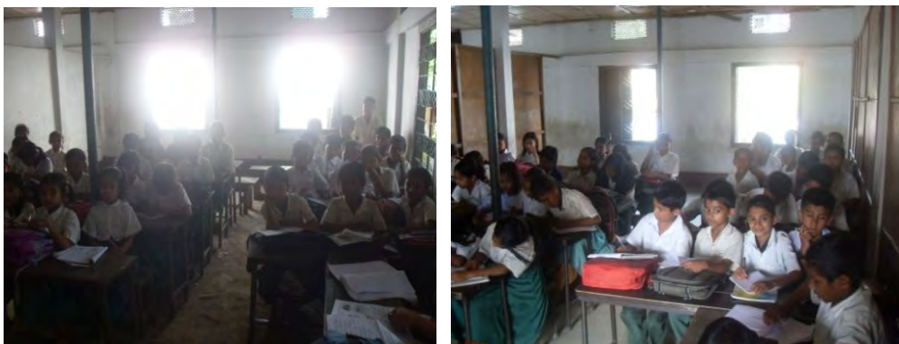
Figure 1.4 Improper direction of daylight causes an unfavorable luminous condition in the classroom at KASDOBIR GOVERNMENT PRIMARY SCHOOL)
