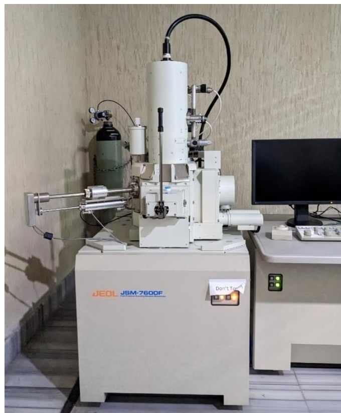
Figure 9: Field Emission Scanning Electron Microscope (FE-SEM: JEOL JSM 7600F)
