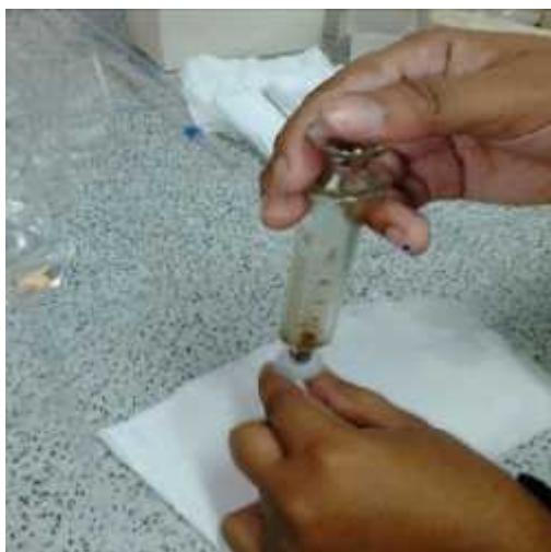
A. Sample passed through microfilter to remove any tiny particle
