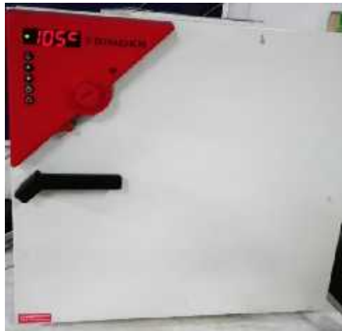
B. Drying samples for 8-10 hours at 102°C
