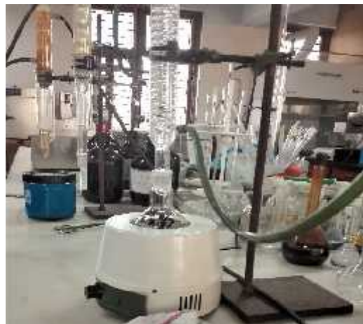
B. Sample in the heating mental for hydrolysis
