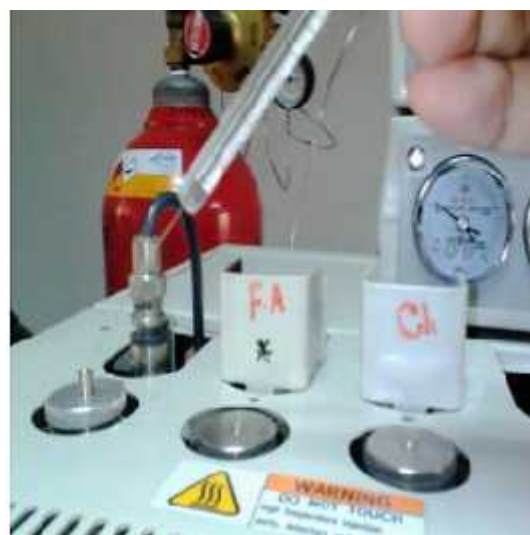
D. Injecting (0.2-0.3) \mu l sample in injection pore of GC
