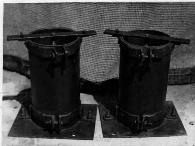
Fig. 4.8. Mold for tensile bond strength test specimen.
