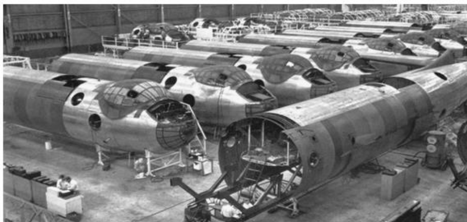
Figure 2.13 US Air Force's B-36 Long-range Bombers Assembly Line (Dark looking Mg sheet in the picture) [87]
