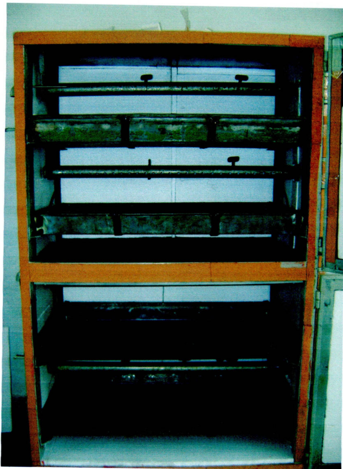
Fig. 3.14: Assembly of the dryer chamber
